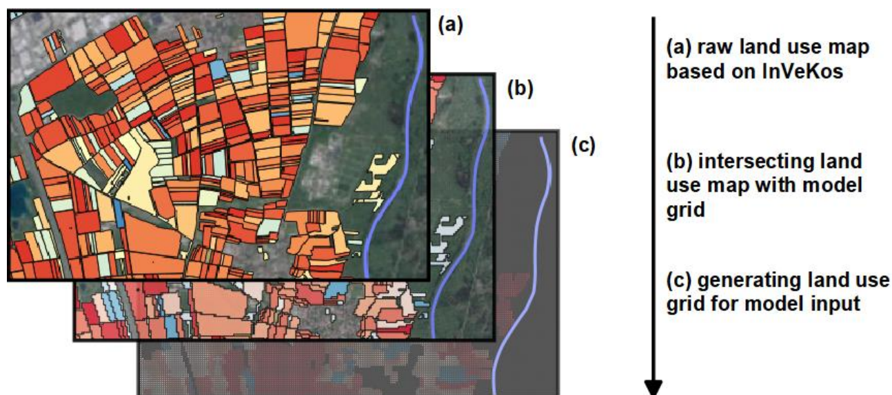
Figure 4: Implementation of InVeKos land use data (LfL, 2018) into the hydrologic model, example scheme as implemented for the land use in 2012.
