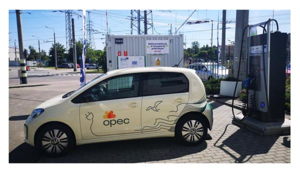
The City of Gdynia and the <u>trolleybus operator PKT</u> have completed two EU projects by implementing and testing an innovative solution, a mobile charging station for electric cars, powered by the trolleybus network. Within the Interreg EfficienCE project an energy storage inverter has been designed and constructed by PKT, which is a device for processing excess braking energy and traction power.
