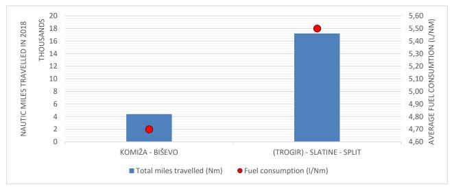
Figure 29 Passenger boats miles vs. average fuel consumption
