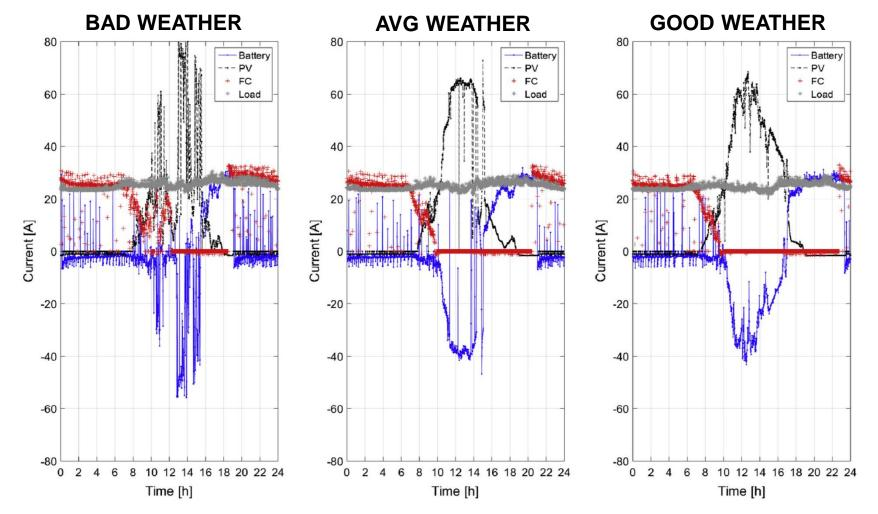
Fig. 9. Current output of PV system, battery, Fuel Cell and load during three representative days in the month of September 2015, Fiano Romano site (#2). from Cordiner, Mulone et al., Applied Energy, 192, 2017
