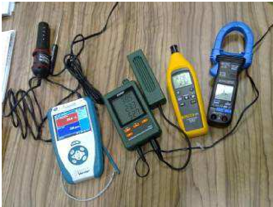
Figure 1: Some instruments for the measurement of living comfort and energy consumption at energy audit in building
