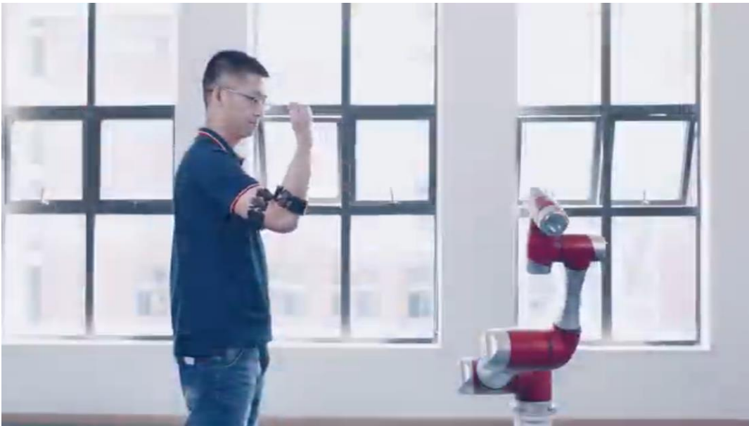
Figure 10: Robot control through motion transmission (Source: JAKA Cobot)
