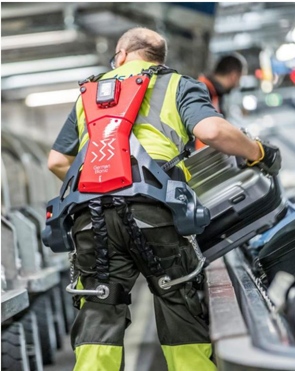
Figure 03: Exoskeleton to support lifting operations (Source: German Bionic)
