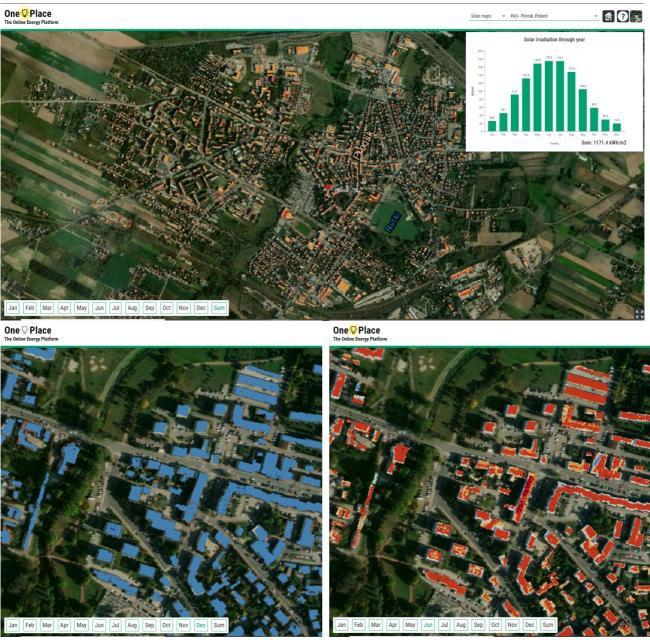
Figure 15. Plonsk municipality (Poland) – Overall solar irradiation per year (above) and photovoltaic PV maps in December (lower left) and June (lower right).
