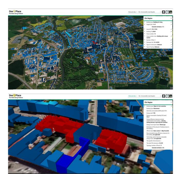
Figure 5. Generated 3D building models for PA3 – Zlin, Czech Republic (PP3), Kromeriz municipality.
