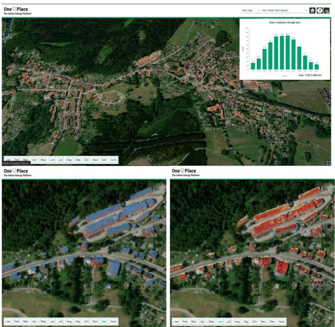
Figure 17. Poland / Czech Republic crossborder region (example of Zacler, CZ) - photovoltaic PV maps in December (on the left) and June (on the right).
