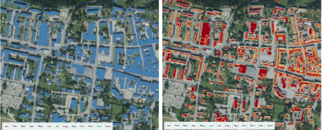
Figure 13. Judenburg-Lindfeld municipality (Austria) – Overall solar irradiation per year (above) and photovoltaic PV maps in December (lower left) and June (lower right).
