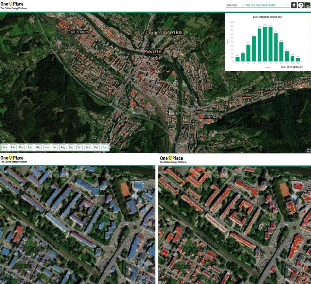
Figure 14. Zlin region – Vsetin (Czech Republic) – Overall solar irradiation per year (above) and photovoltaic PV maps in December (lower left) and June (lower right).
