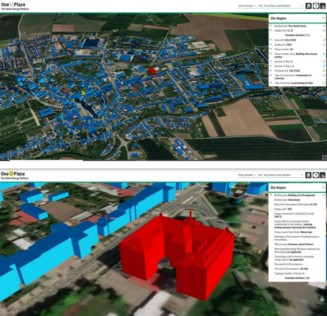
Figure 6. Generated 3D building models for PA3 – Zlin, Czech Republic (PP3), Holesov municipality.
