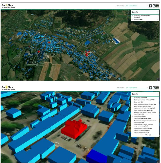
Figure 12. Generated 3D building models for PA8 – the CZ-PL cross-border region (PP12) -Lubawka municipality.
