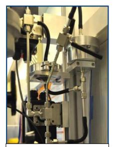
Functional control unit at the Scanning Mobility Particle Sizer (SMPS) in Chernivtsi and Dresden. Source: www.ufireq-central.eu
