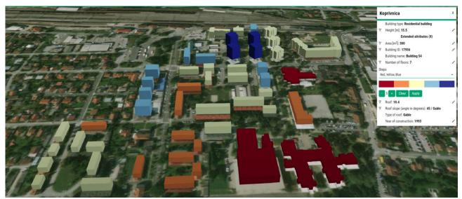
Figure 6: Example of aggregation functions within 3DEMS – number of floors. Source: OnePlace platform presentation
