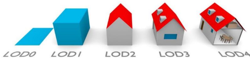
Figure 25: Different Level of Detail (LoD) in 3D building models (source: TU Delft)
