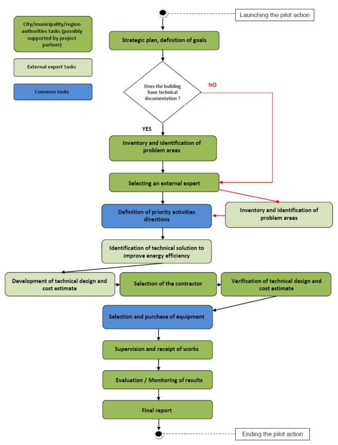
Figure 3: PA3 implementation procedure diagram.
