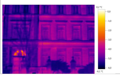
After the lowering the night temperature and change of the windows the heat losses decreased and the frames of the windows are much colder.
