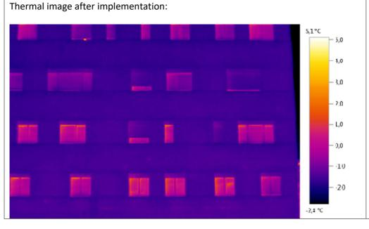
Building is completely insulated with no visible heat losses. The windows are warmer because of the artificial light inside. It wasn't possible to switch off all lights in the hospital.
