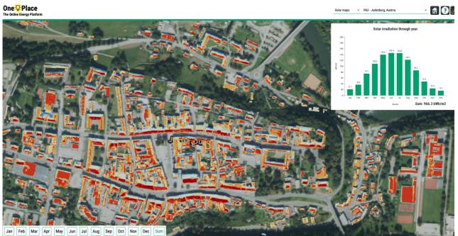
Figure 2: Photovoltaic (PV) potential of building roofs displayed per month and as a yearly sum.
