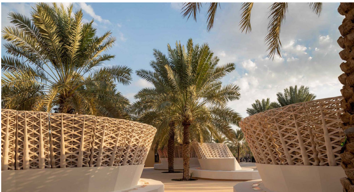
Arthur Mamou-Mani's Sandwaves is the largest sandprinted installation yet, it consists of 58 3D-printed elements.
