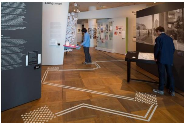
Figure 17: Tactile control system
