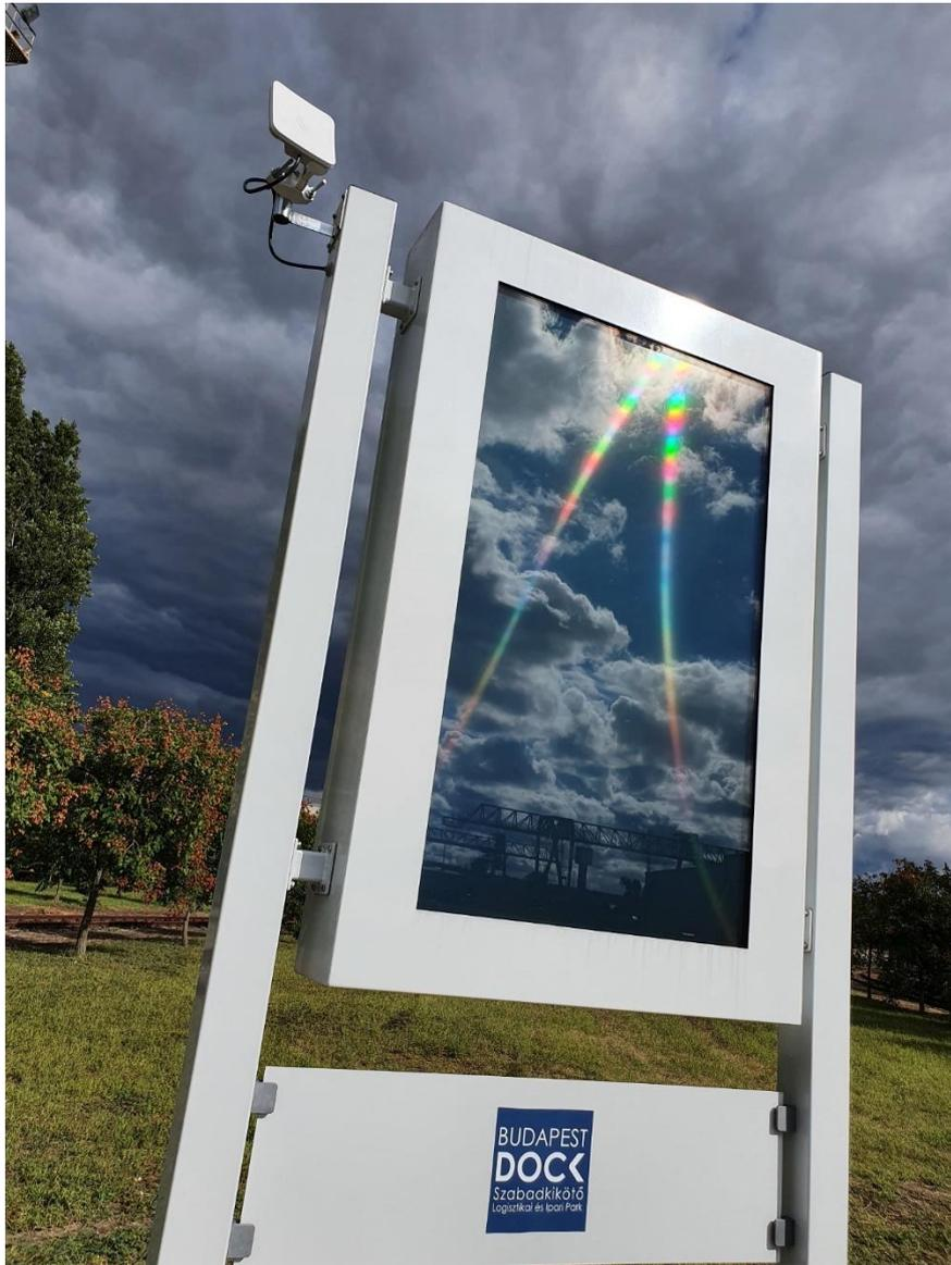
The screens were designed specifically at the request of the FBL. They are Wi-Fi connected to the core system and the license plate recognising cameras detect the vehicle and drives the instruction for navigation to screen upon approaching the destination.
