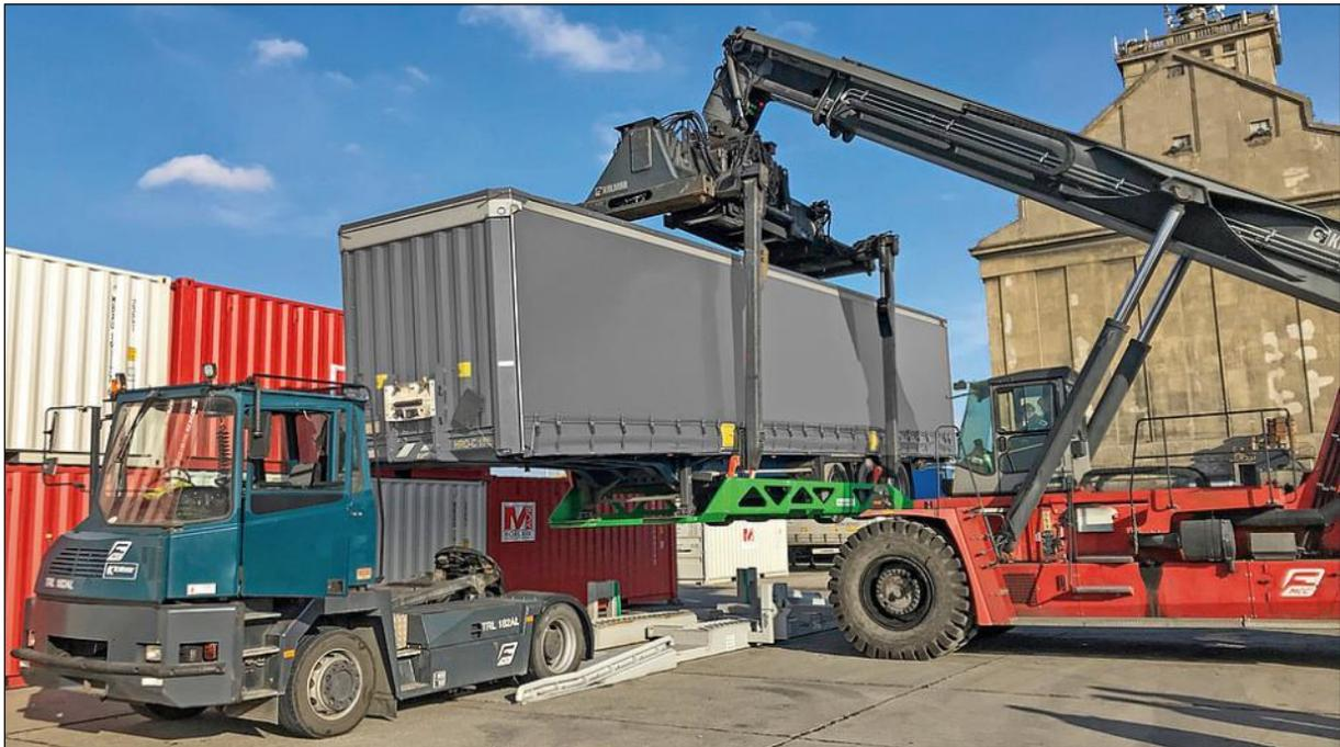
Figure 6: Loading system NiKRASA in the MAHART intermodal terminal in Budapest (source: [www.dvz.de](http://www.dvz.de))
