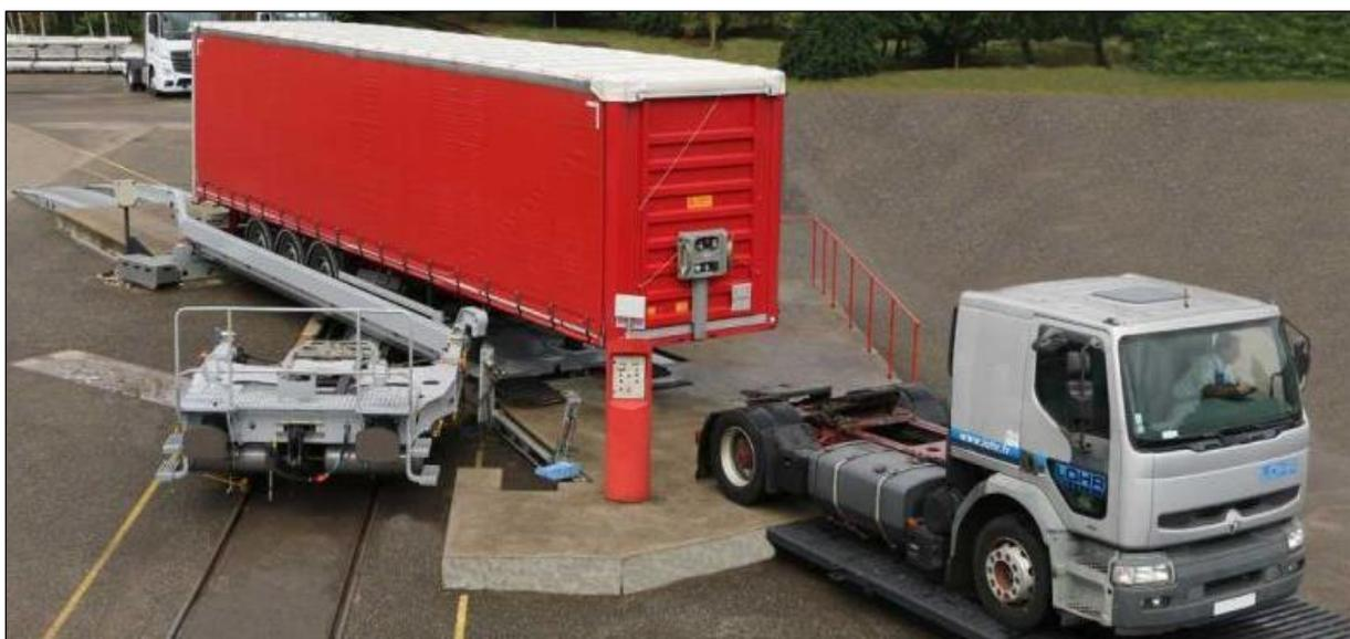
Figure 11: LOHR railway system
