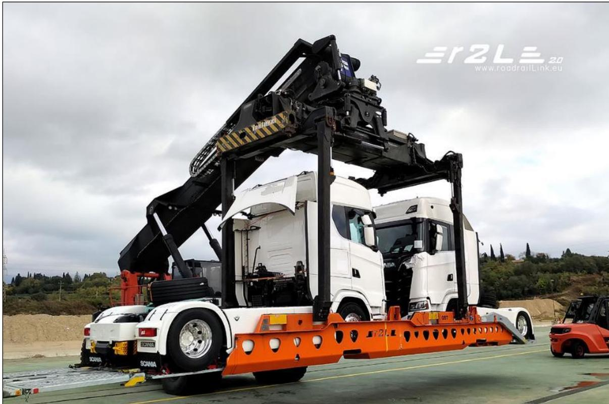
Figure 8: handling of lorry tractors with VEGA equipment
