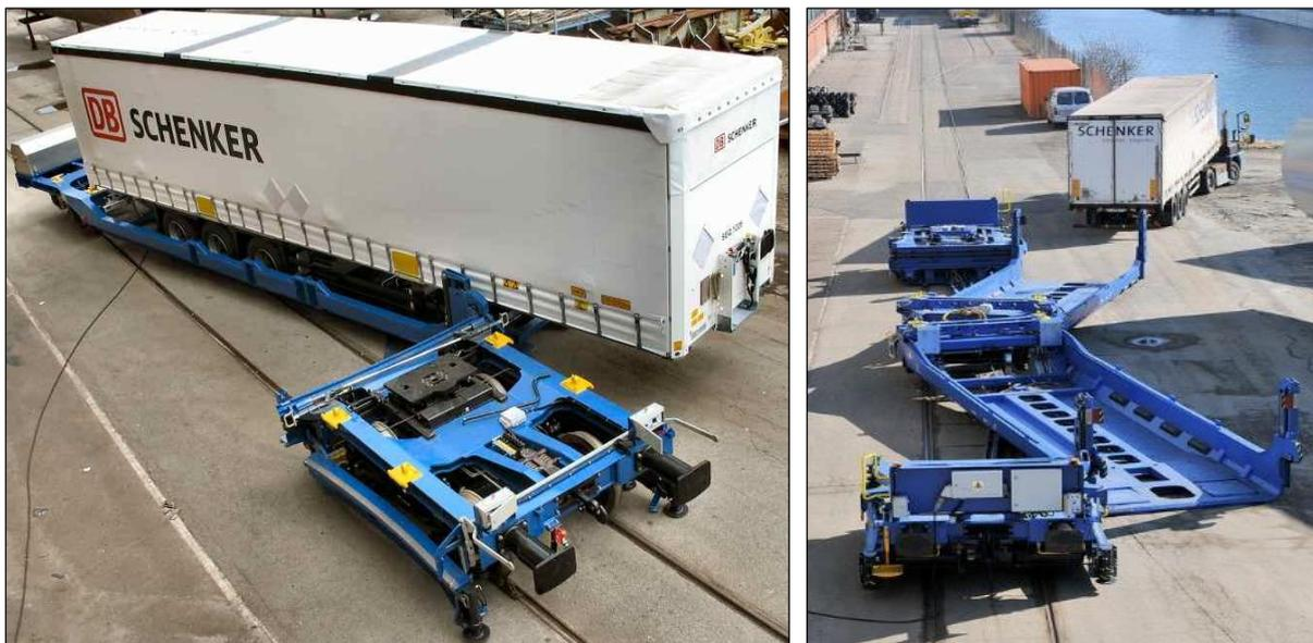
Figure 14: system Megaswing: loading process
