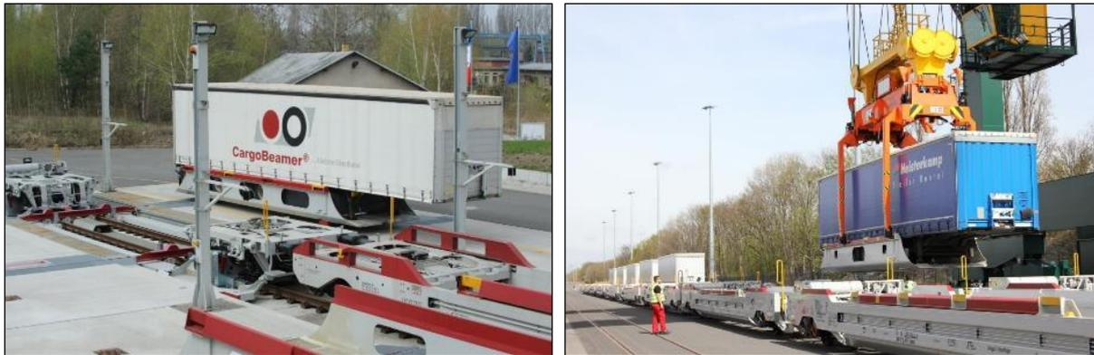
Figure 9: system CargoBeamer<sup>2</sup>: horizontal (left) and vertical (right) handling
