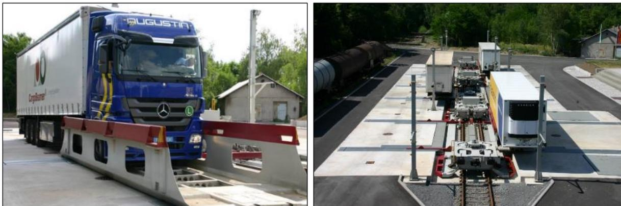
Figure 10: truck enters the transport tray (left), test terminal in Leipzig (right)
