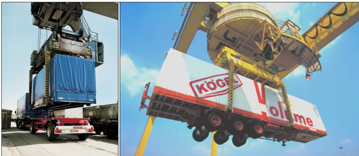
Figure 4: Bottom lifted swap bodies (left) and semitrailers
