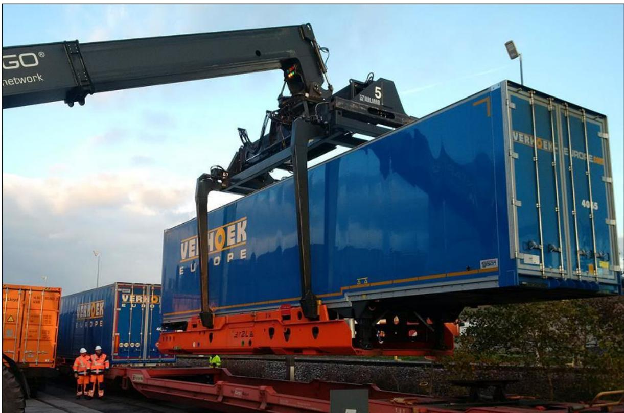
Figure 7: Loading system VEGA (source: [www.roadrailink.eu](http://www.roadrailink.eu))
