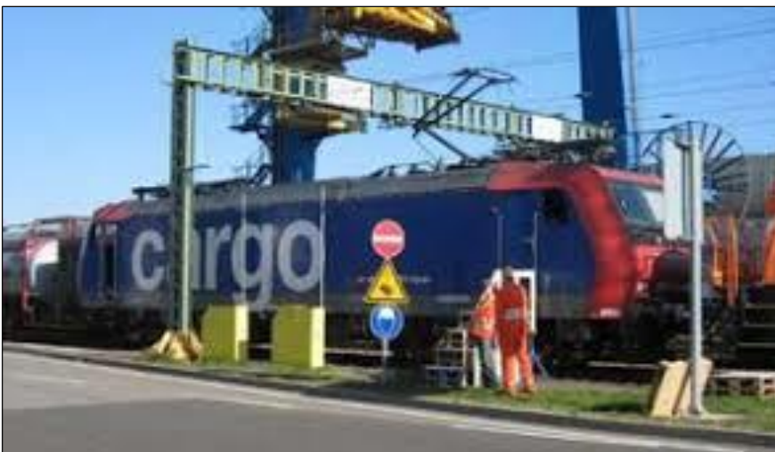
Figure 10: Electric locomotive in a terminal with electrified end sections of transshipment tracks. The front part of the locomotive is still in the electrified section, with one pantograph lifted to the overhead wire, while the rear part of the locomotive is already in the non-electrified section. (Photo: Sondermann/KTL)
