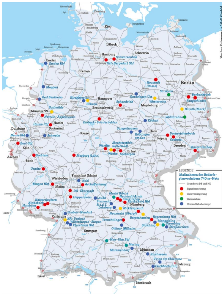
Figure 5: The program for 740 m train length in Germany is an example for how a combination of several small-scale low-cost measures can lead to major improvements in a larger network. On the left side the individual locations and measures enabling the operation of 740 m long trains are indicated (by type of measure: red: moving of signals; yellow: siding extension; green: new track; blue: modification of track layout in stations (Source: VDV). On the right side the networks on which the operation of 740 m long trains in 2020 respectively 2026 will be possible are indicated; further extension of the network is foreseen beyond 2026 (Source: DB Netz). As can be seen, relatively few measures will allow a considerable extension of the 740-m network and ensure continuity of the 740 m-availability in several important corridors, i.a. in German sections of the Orient/East-Med- and Rhine-Danube Rail Freight Corridors.
