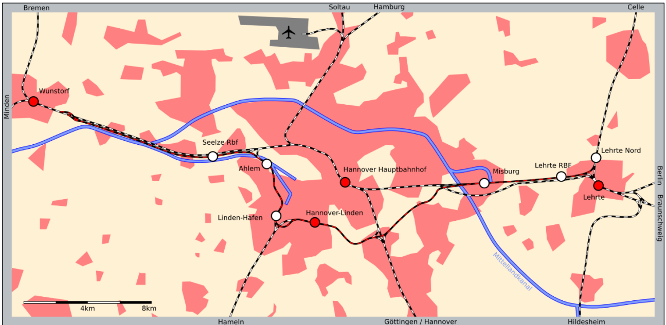
Figure 14: Freight bypass in the node of Hanover in northern Germany. The double-track bypass was opened in 1909, runs mostly on an elevated embankment and connects to several railway lines radiating from the city. (Source: Wikipedia)
