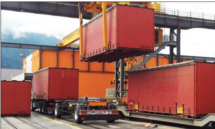
Figure 12: Gripping pliers transhipment of a swap body 5
