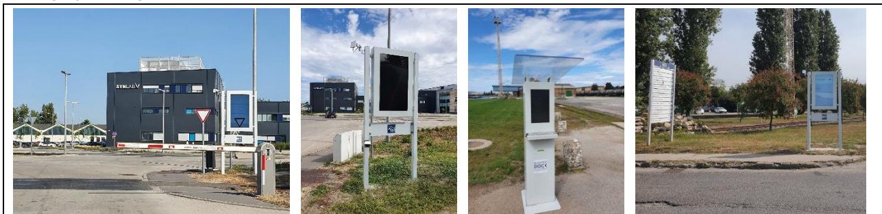
Elements of the smart traffic management system: Access control at the gates, smart info panel with license plate recognition camera, InfoPoint (kiosk) and smart signpost (source: FBL)
