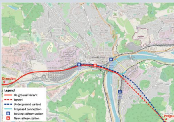
Main station in Ústí nad Labem and planned railway lines with proposed additional connection
