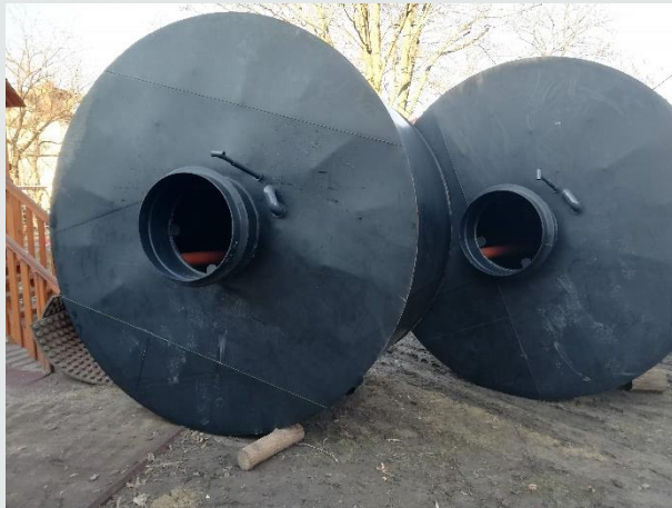
Water tanks (2 x 7 m3)
