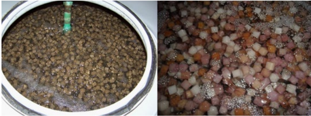
Figure 13: Aerated moving-bed biofilm reactor (MBBR) (left) and foam cubes as carrier media (Photo: E. Nolde).
