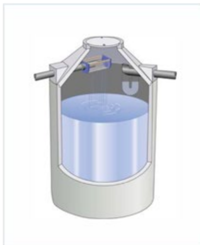
Underground concrete cistern (3 - 12 m 3 ) (Mall)
