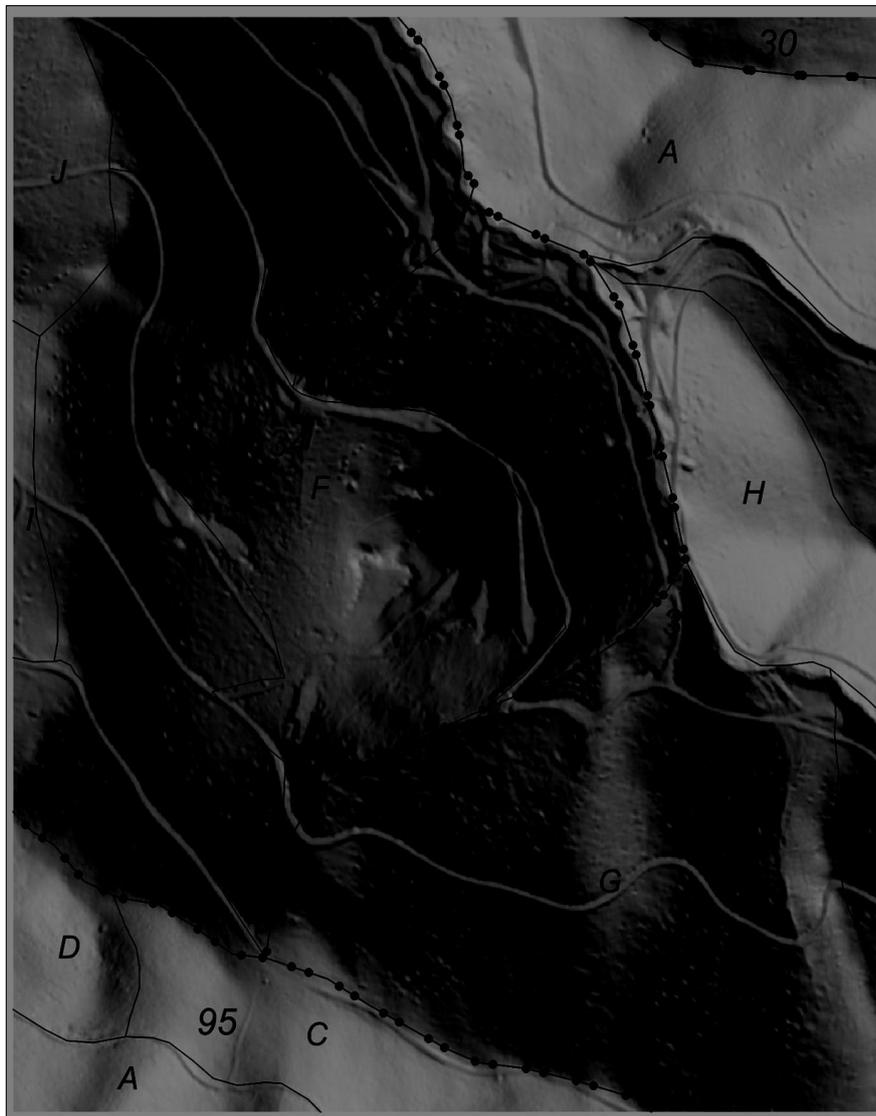
Figure 3.: R: erosion caused by skidding in the Királyháza area. L: fragmentation caused by intensive forest road system in the Kuruc-creek valley
