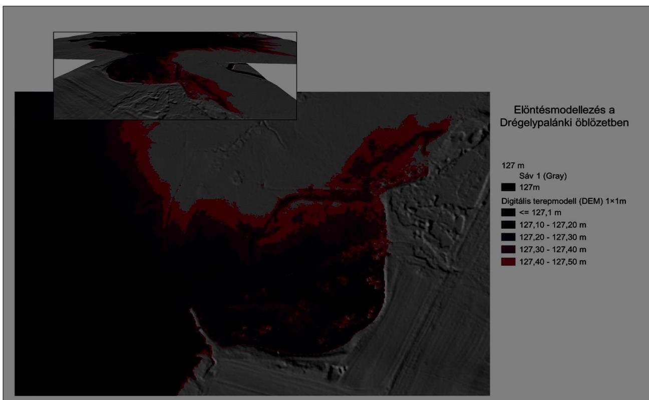
Figure 4: Flood modeling on a small „side-basin”. The vertical resolution is 10cm. The deeper and higher ground can be easily identified, therefore the ideal direction of the flooding is readable
