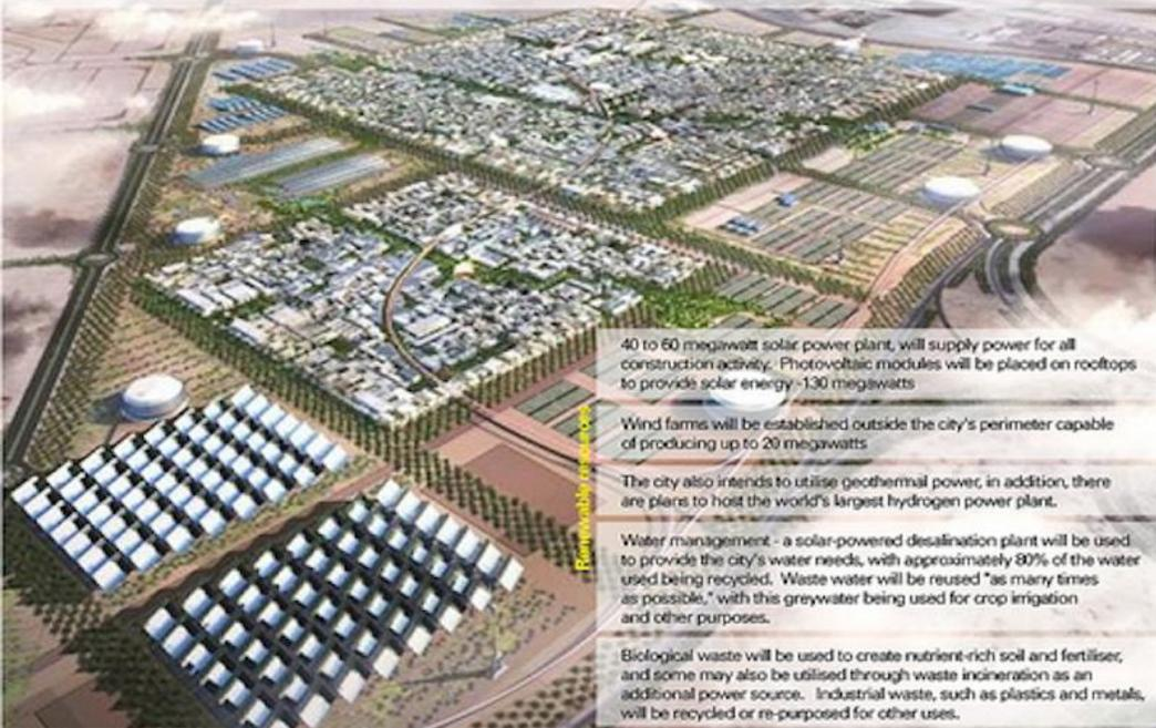
40 to 60 megawatt solar power plant, will supply power for all construction activity. Photovoltaic modules will be placed on rooftops to provide solar energy -130 megawatts
