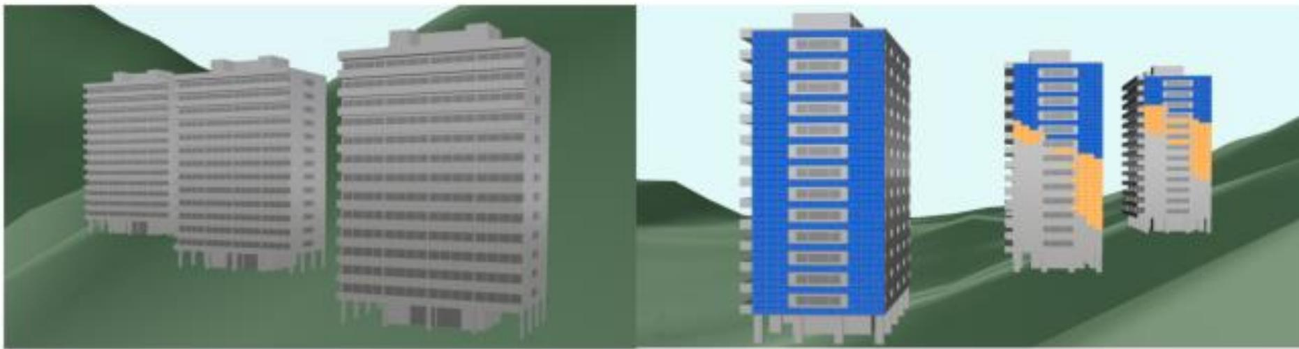
3D representation of the three high rise buildings; (right) representation of the BIPV plant with two optimal NPV solutions: if the cost of storage is 1000 €/kWh no battery is installed and the plant is limited at the blue area. If the cost of storage is 250 €/kWh, 87 kWh of batteries are installed allowing a larger BIPV plant (orange area).
