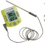
FIGURE 7: Example of a digital thermometer to be used for the manual monitoring of temperature in the chosen classroom.
