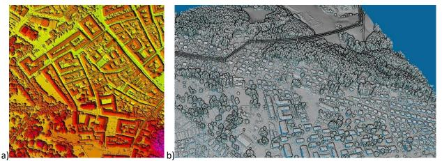
*Figure 4: Example of photogrammetric point cloud derived from aerial images (a – source: FBK) and acquired with airborne laser scanning / LiDAR (b – source: Municipality of Velenjie).*
