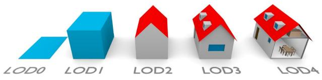
Figure 1: Different Level of Detail (LoD) in 3D building models (source: TU Delft).
