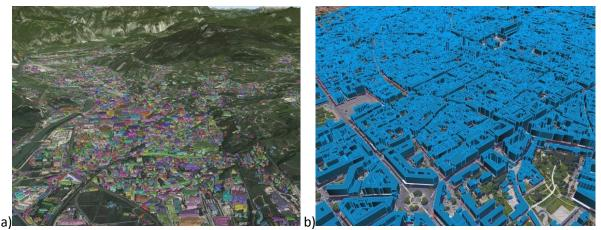
*Figure 8: LoD1 over the city of Trento (a) and Bologna (b) generated extruding the available vector building footprint to a given height stored in the attributes of the vector data (source: FBK).*
