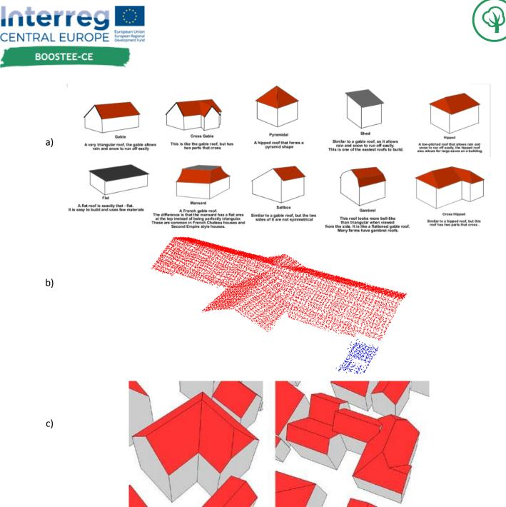
Figure 7: Example of roof primitives (a) which are then fitted onto roof point clouds (b) to derive LoD1 or LoD2 (c) building models (depending on the density of the point cloud and complexity of the roofs).
