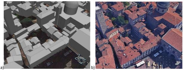
Figure 6: 3D building geometries (LoD2) derived fitting geometric primitives on point clouds (a: source: FBK) wrt polygonal mesh model (b: source Google Earth).
