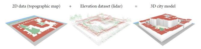
*Figure 9: An hybrid approach to generate 3D building models: building polygons/footprints are extruded up to the height provided by a DSM (e.g. acquired with LiDAR)*
