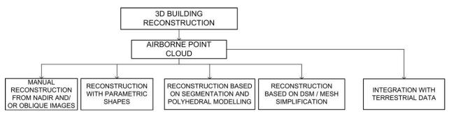
Figure 5: 3D building geometries from airborne point clouds: various methods to derive 3D gemetries, e.g. through manual reconstruction, using parametric shapes, based on polyhedral modeling or applying a mesh semplification. Often terrestrial 3D data al also integrated..
