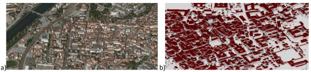
*Figure 2: Different representation of a 3D city model: large and unique polygonal model with texture (a – source: FBK), single polygonal models in LOD2 (b – source: FBK).*
