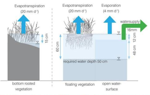
Fig. 34: Water level fluctuation in a CSW during a 30 day drought with bottom rooted vegetation (left) and floating mats with macrophytes (right) (Günther, 2013, p.25)
