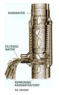
A downpipe filter collector diverts 90% of the rainwater to a storage tank through a 0.17 mm stainless steel mesh filter A floating fine suction filter ensures that rainwater is pumped from cleanest level of the tank and is free of particulates A large vortex fine filter diverts 90% of rainwater runoff from roof areas of up to 500 m<sup>2</sup>
