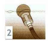
A floating fine suction filter ensures that rainwater is pumped from cleanest level of the tank and is free of particulates
