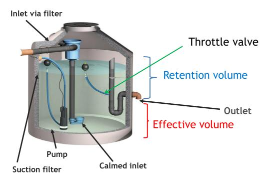
A conflict exists between rainwater utilisation (cistern should be full at all times) and the hydraulic relief of sewer (cistern should preferably be always empty, in order to collect new runoff). Retention cisterns are constructed as a combination structure to fulfill both demands. They have a specific **retention volume**, which can be throttled discharged into sewer and an additional fixed **effective volume** for reuse.
