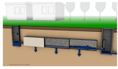
Schematic diagram of an infiltration trench with a sedimentation chamber at inflow and throttled outflow (Source: Sieker)
