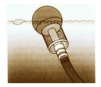
A floating fine suction filter ensures that rainwater is pumped from cleanest level of the tank and is free of particulates
