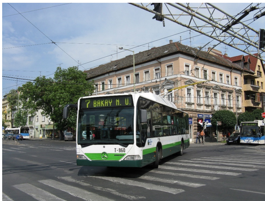
Figure 6: A converted trolleybus of SZKT in Szeged [Photo by SZKT Szeged]
