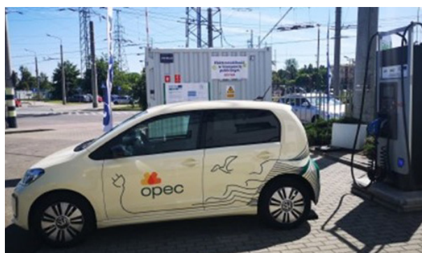
Figure 6: Mobile charging station for electric cars powered by the trolleybus network (PKT)
