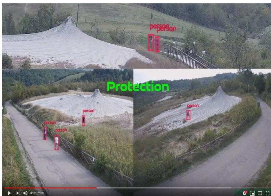
Fig. 10 - Testing phase of the system. Combination of the views of the three cameras, with the recognition of people walking on the street and invading the Zone A of the Natural Reserve, beyond the fences. From the entire explanation video .
