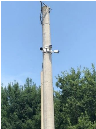
Fig. 6a,b - ENEL concrete pole with the three cameras installed (a) and monitoring equipment in Cà Rossa: the industrial PC is the small box with the label Vision-e, on the top right of fig 6b.
