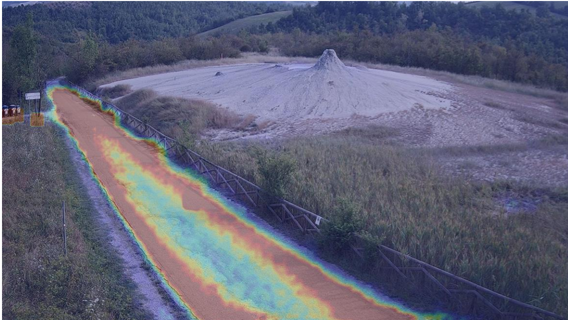
Fig. 18 - General HeatMap. As expected, the flow of vehicles and pedestrians, saturates the information along the municipal road. In any case it can be noted the splitting in two main parts, related to the go/back flows.
