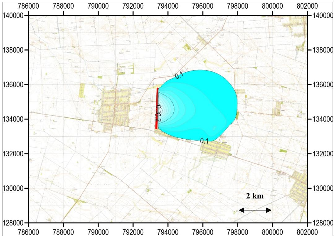
Figure 32. Groundwater level rise (m) in the second aquifer due to the effect of the underground dam
