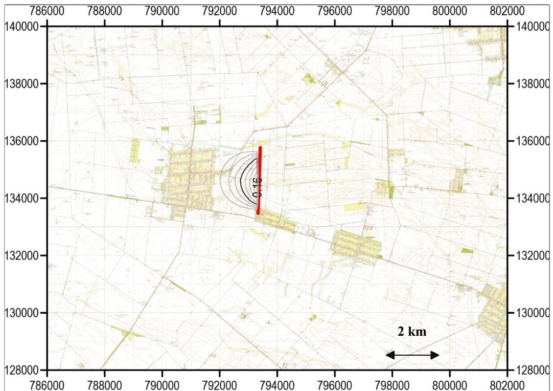
Figure 33. Groundwater level fall (m) in the second aquifer due to the effect of the underground dam
