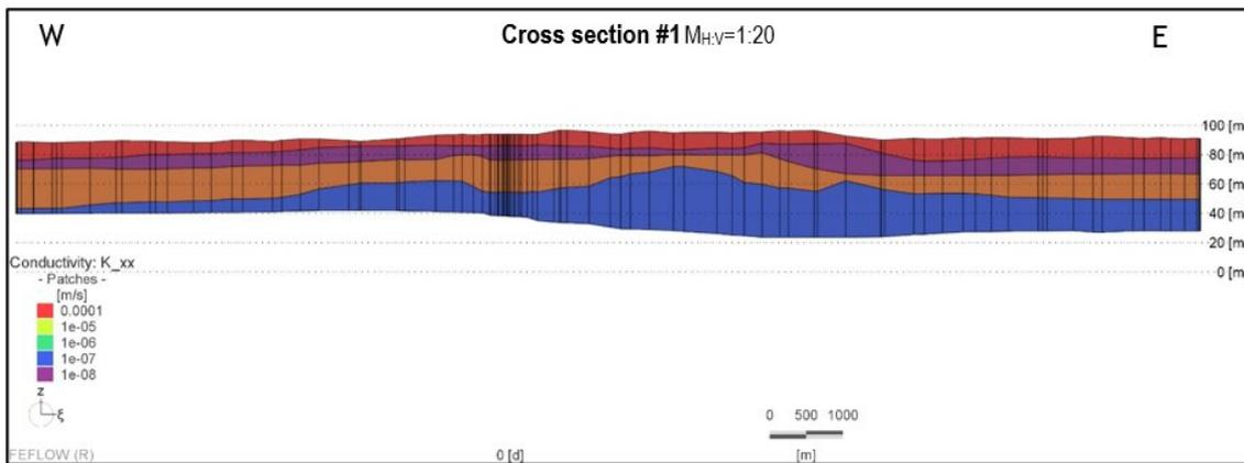
Figure 22. Hydraulic conductivity values used in the model along Section 1.
