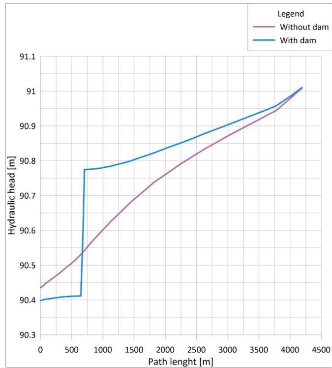
Figure 27. Hydraulic heads as the effect of the emplacement of the underground dam along Section 2.
