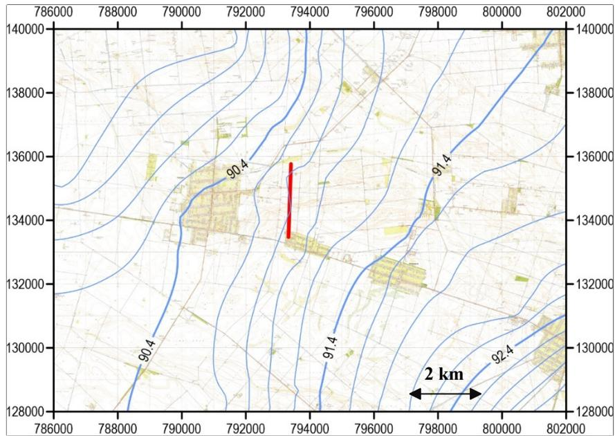
Figure 26. The representation of modelled water levels (m a.s.l.) in the first aquifer (red underground dam)
