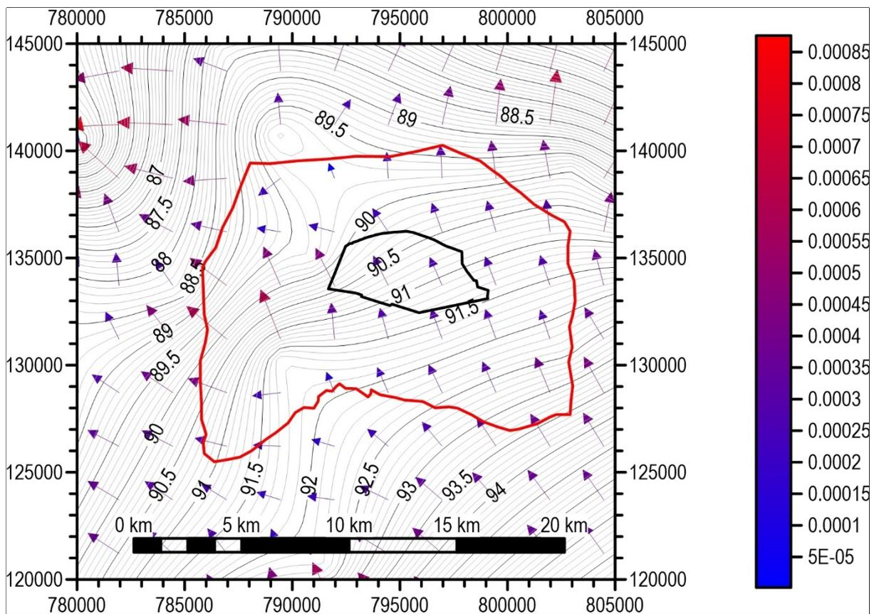
Figure 24. Hydraulic potential and gradient distribution of the static water level (m a.s.l.) used for the modelling
