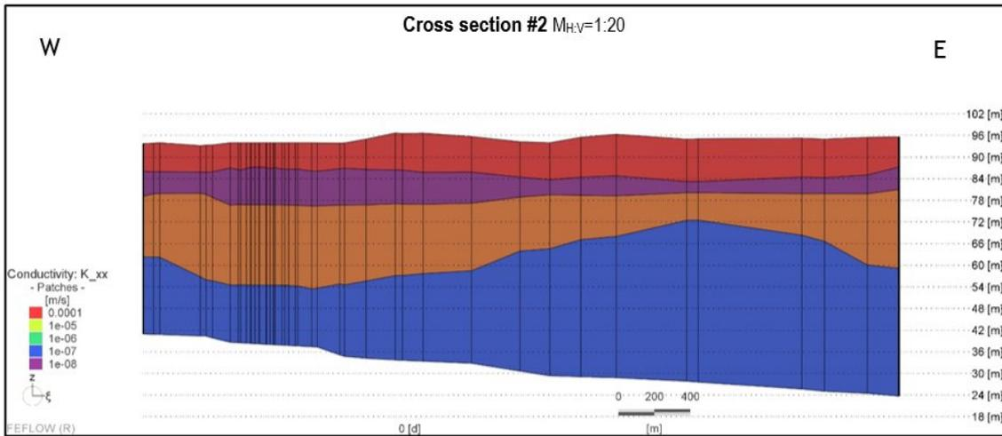
Figure 23. Hydraulic conductivity values used in the model along Section 2.
