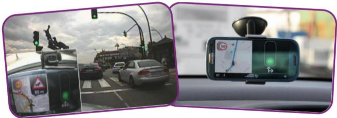
The pictures above show the HMI display combining in a map the RHW and EEIS services, with countdown of the time-to-green or time-to-red at equipped intersections in the city of Vigo.
