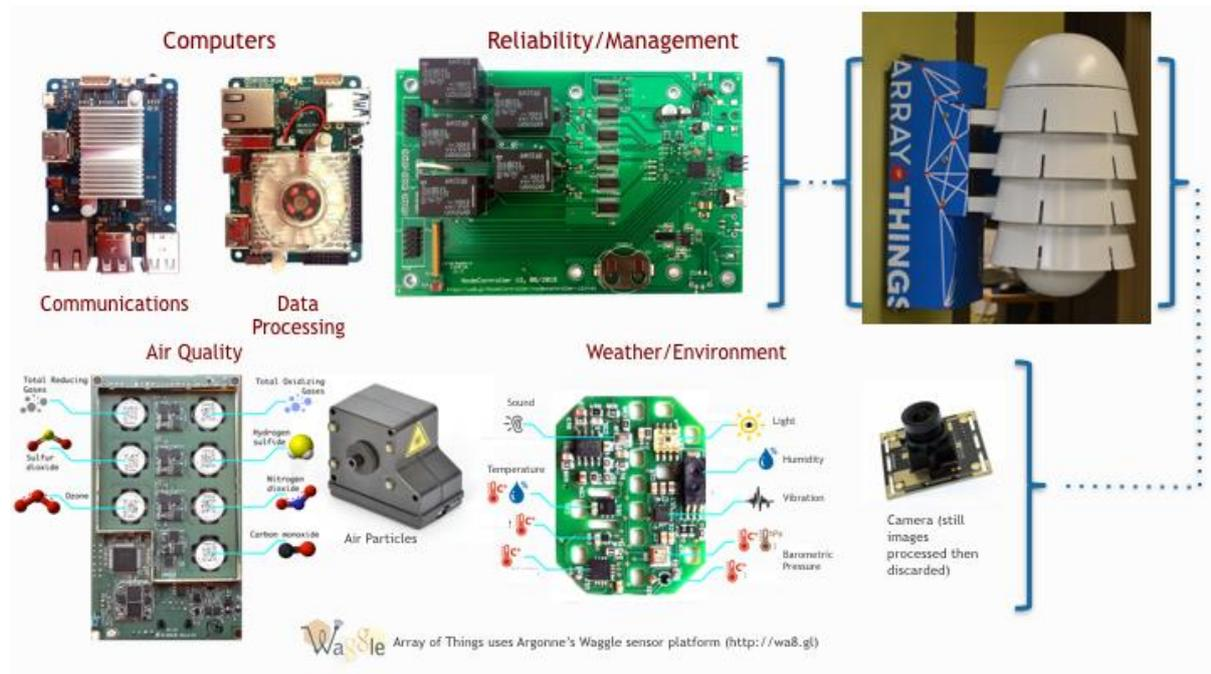
**Figure 14 - Current AoT Node Architecture**
