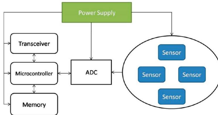
**Figure 5 - The architecture of a Wireless Sensor Node**
