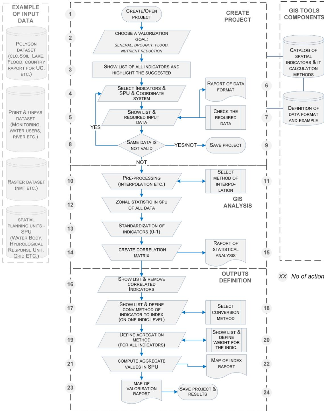
Fig. 2 Algorithm of the GIS tools for valorization of water retention needs (source D.T1.1.1)
