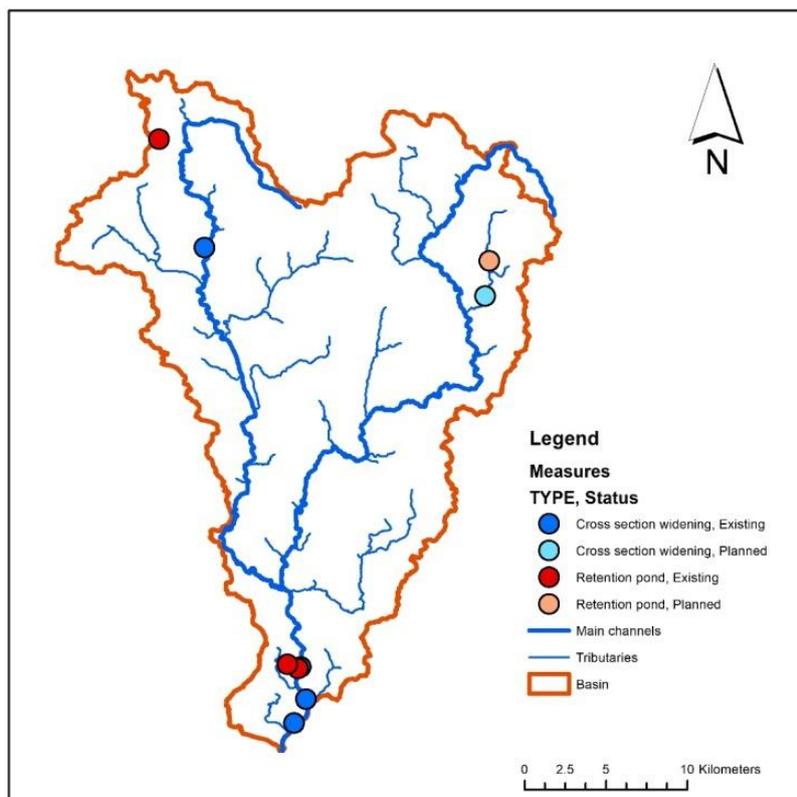
Figure 20: Existing and planned retention measures affecting the sediment issue in the Aist catchment
