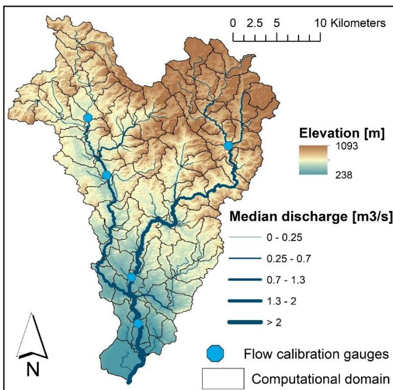
Figure 13: SWAT model computational domain and simulated river network
