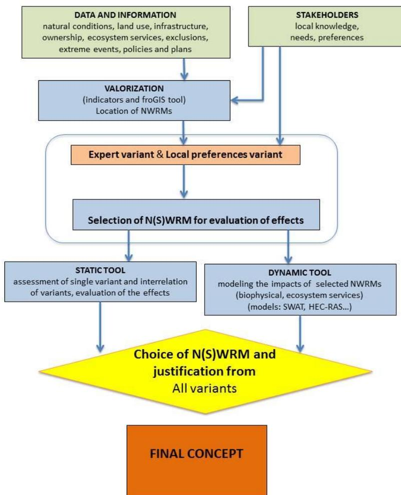
Figure 1. Main steps of the concept plan elaboration
