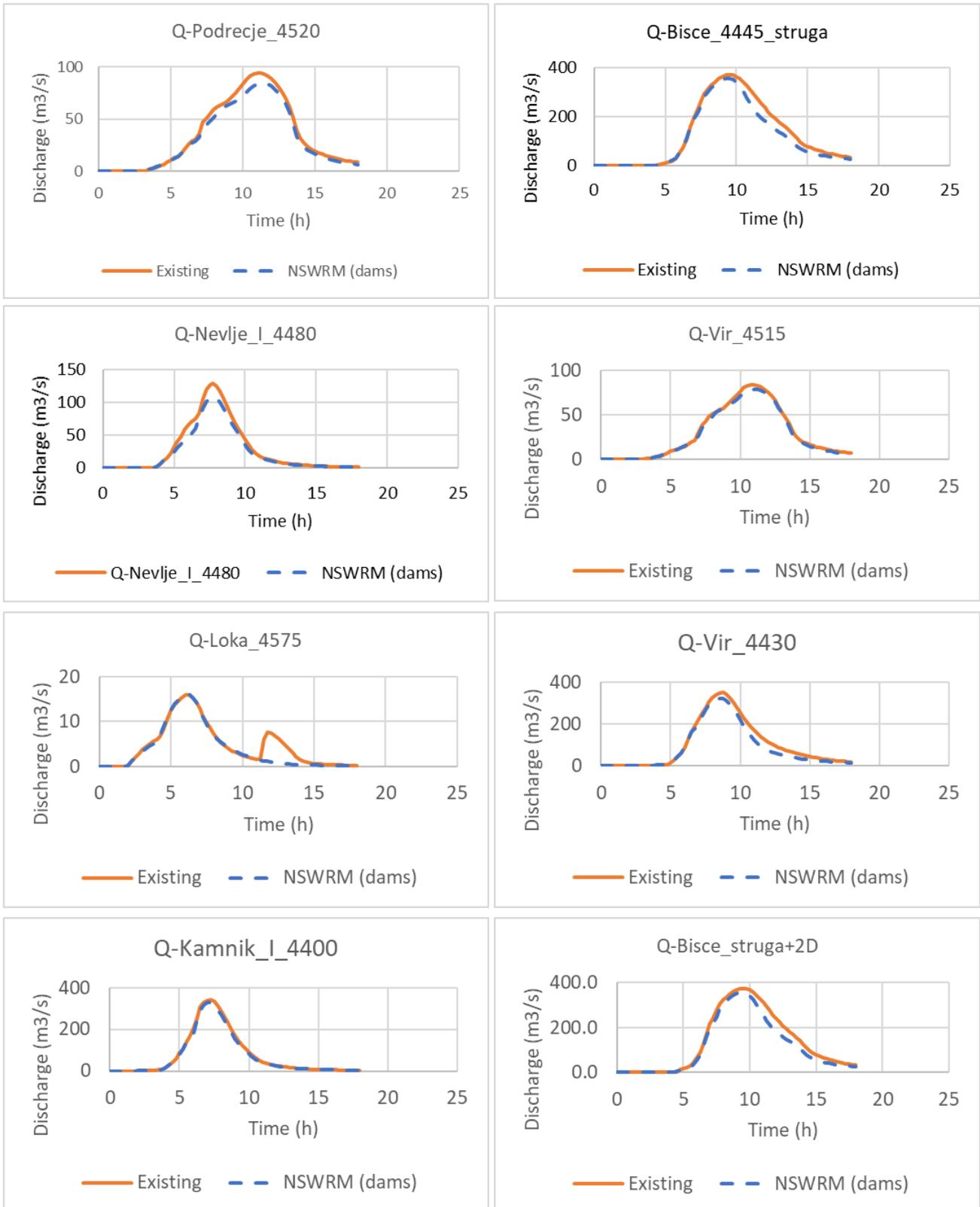
Figure 38: Comparison of computed 6-hour hydrographs with 100-year return period
