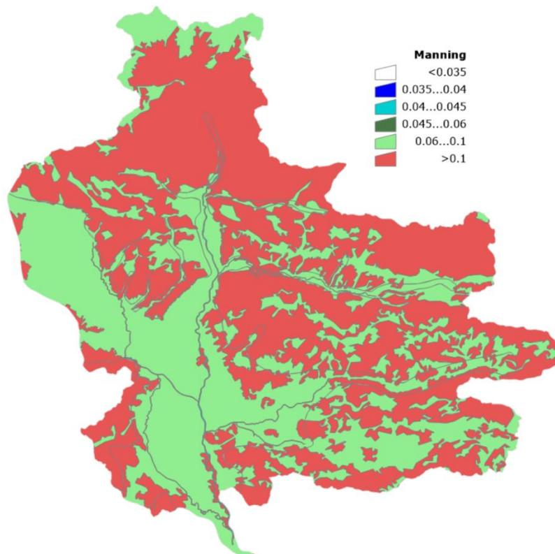
Figure 26: Calibrated values of Manning's roughness coefficient
