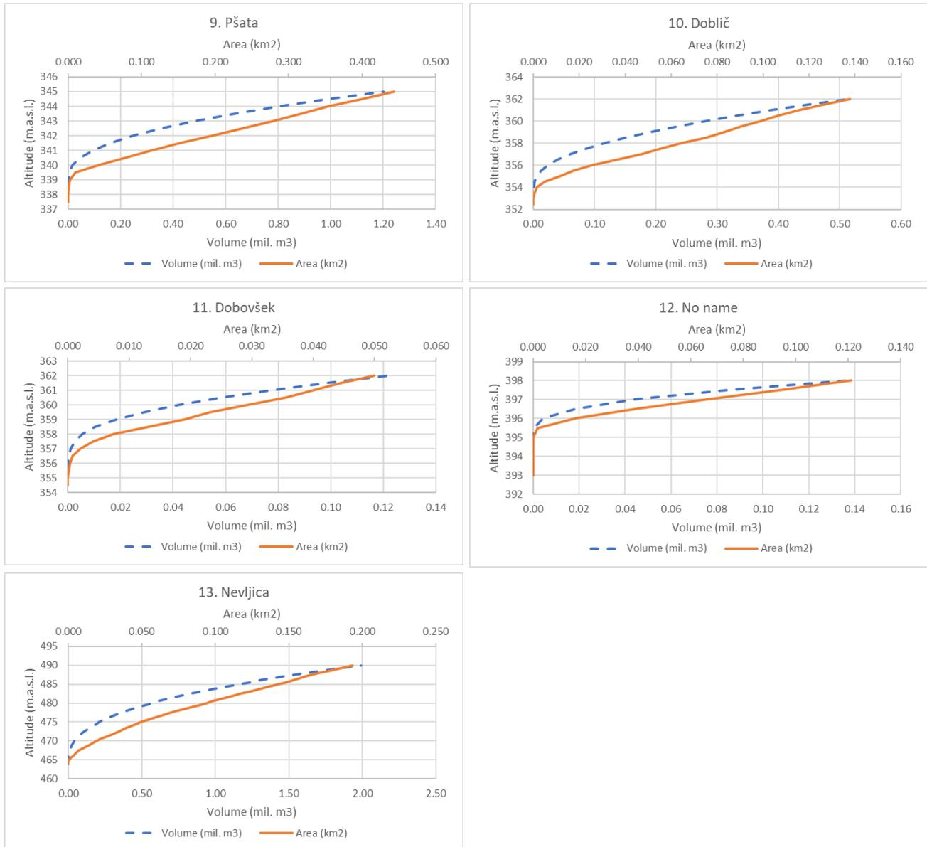
Figure 35: Calculated volume and flooded area for every proposed dam, based on Lidar
