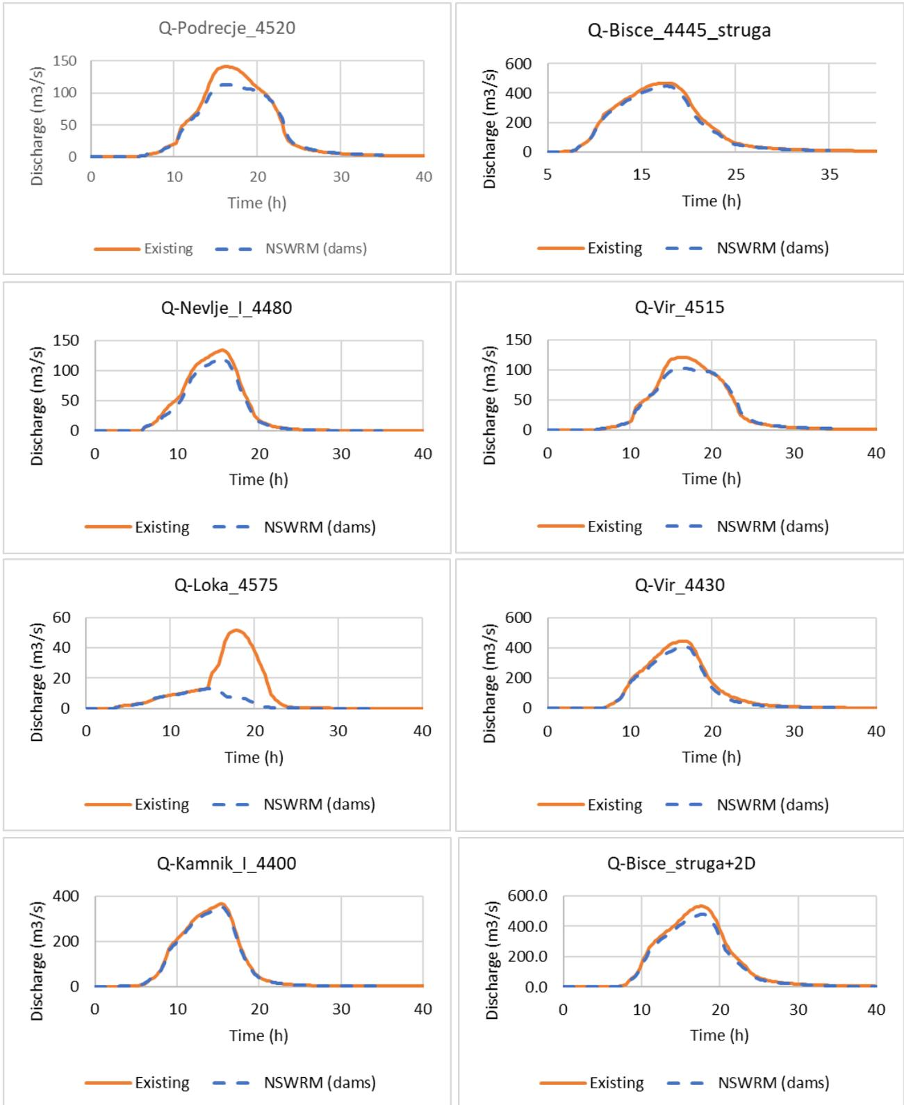
Figure 39: Comparison of computed 15-hour hydrographs with 100-year return period
