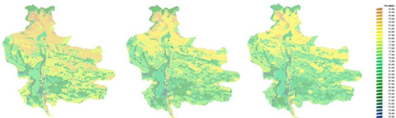
Figure 8: Curve number classification (from left to right: good, average and bad conditions)
