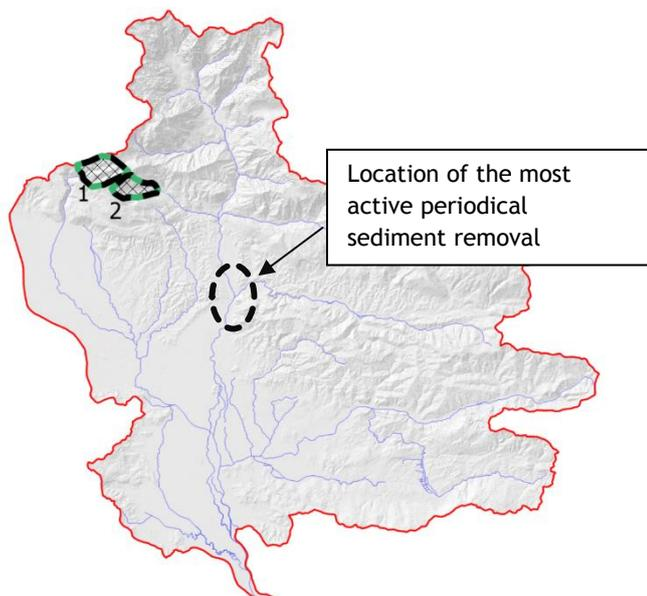
Figure 43: Erosion control measures locations numbering (marked in green-black dashed area)
