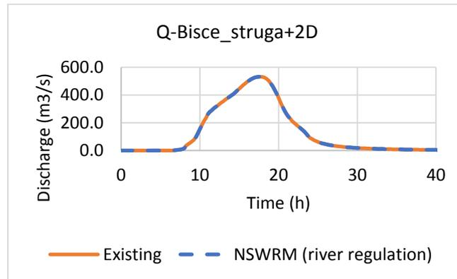
Figure 42: Existing vs river regulation - comparison of computed 15-hour hydrographs with 100-year return period
