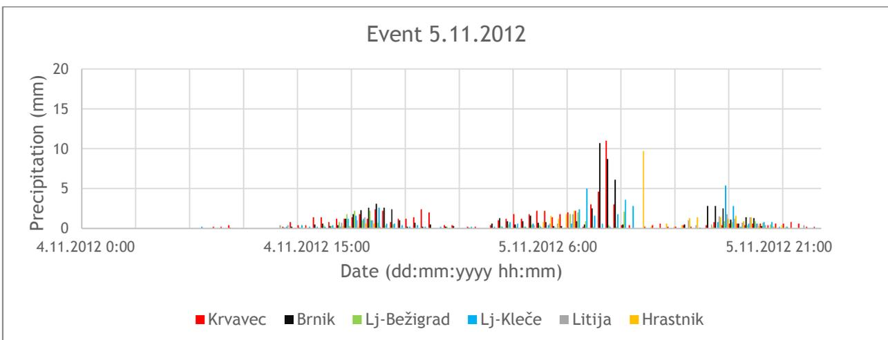
Figure 14: Half-hourly precipitation histogram for the 5.11.2012 event
