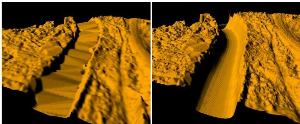
Figure 16: Comparison between raw DEM (left) and modified in-stream DEM (right)
