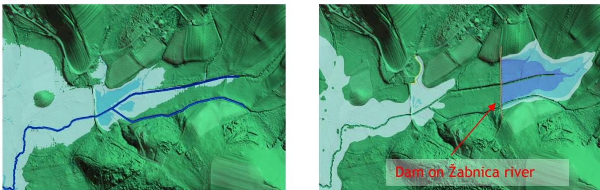
Figure 37: Example - comparison between existing flooding (left photo) and flooding after measures (new dam Nr.3, right photo) on Žabnica river.
