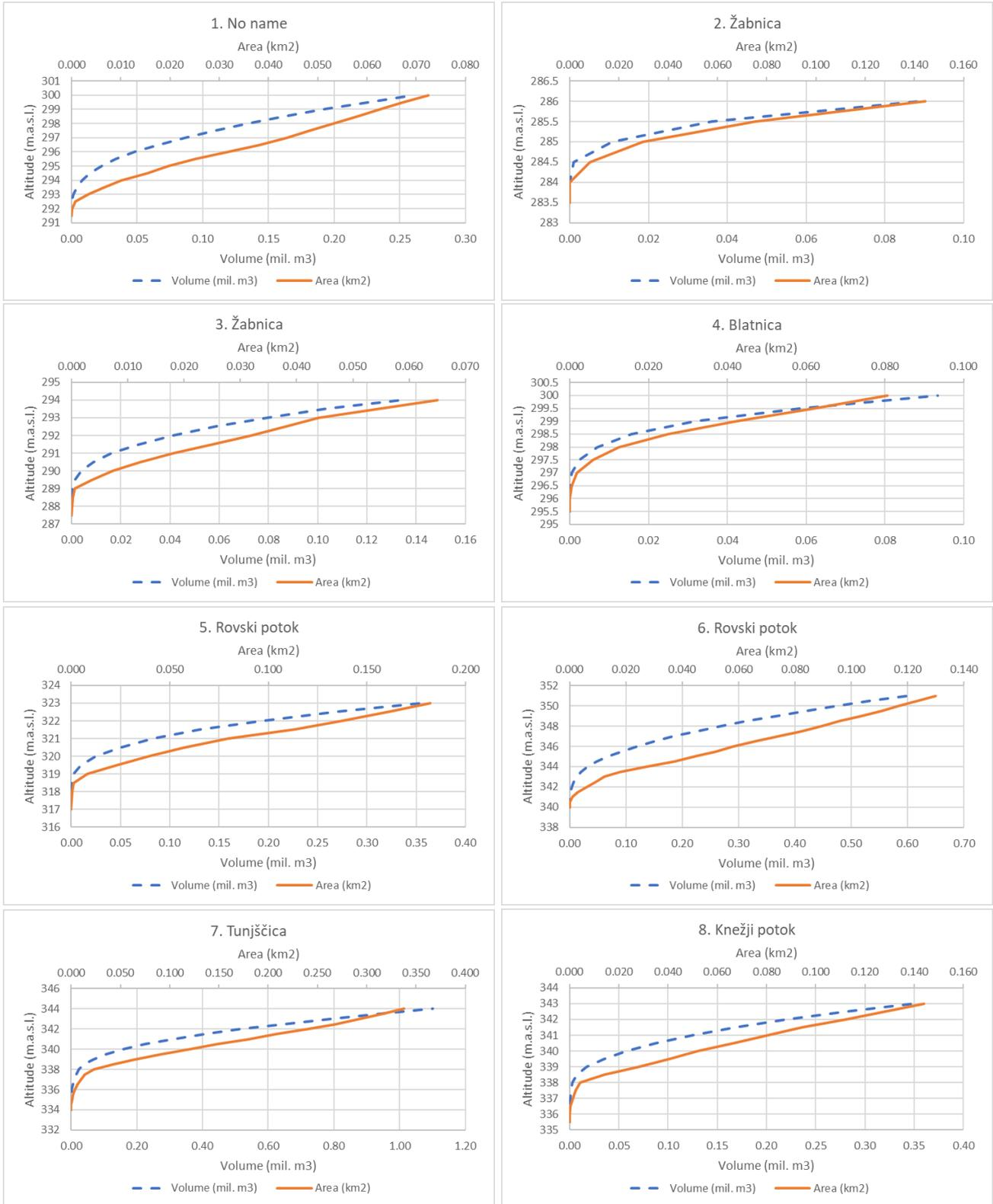
Figure 34: Calculated volume and flooded area for every proposed dam, based on Lidar
