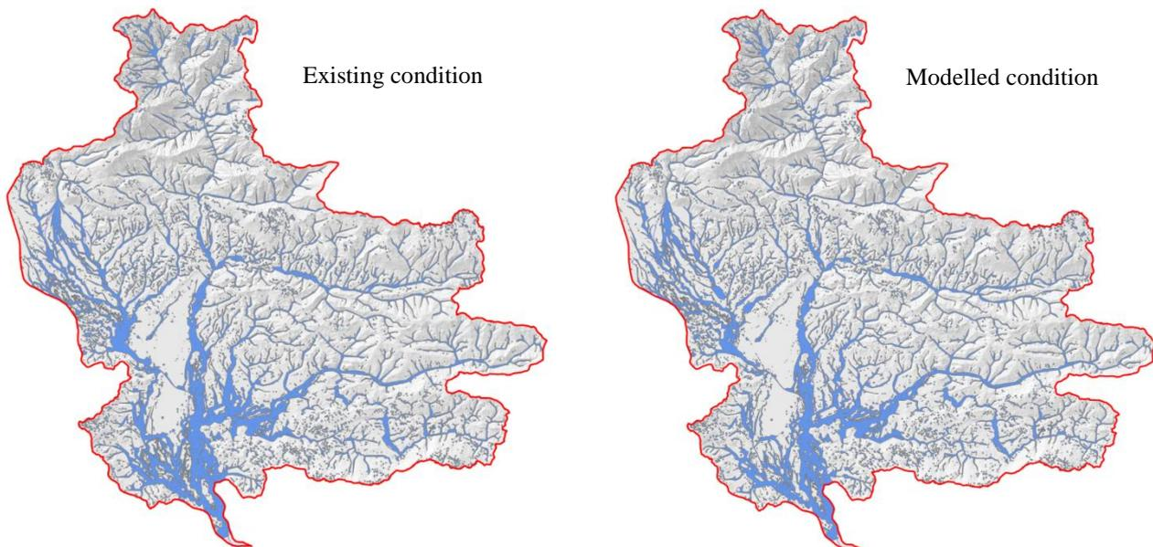
Figure 36: Graphical representation of calculated flooding for 15 hours event with 100year return period. Existing conditions flooding is on the left side, flooding with implemented proposed NSWRM (dams) is on the right. On first look, difference is negligible.
