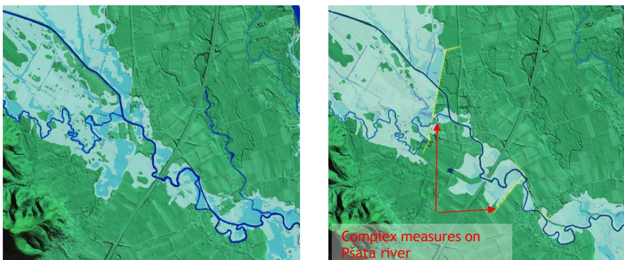
Figure 50: Example - comparison between existing flooding (left photo) and flooding after applying measures (complex measures nr.1,2,3,4,5 and 6, right photo) on Pšata river.
