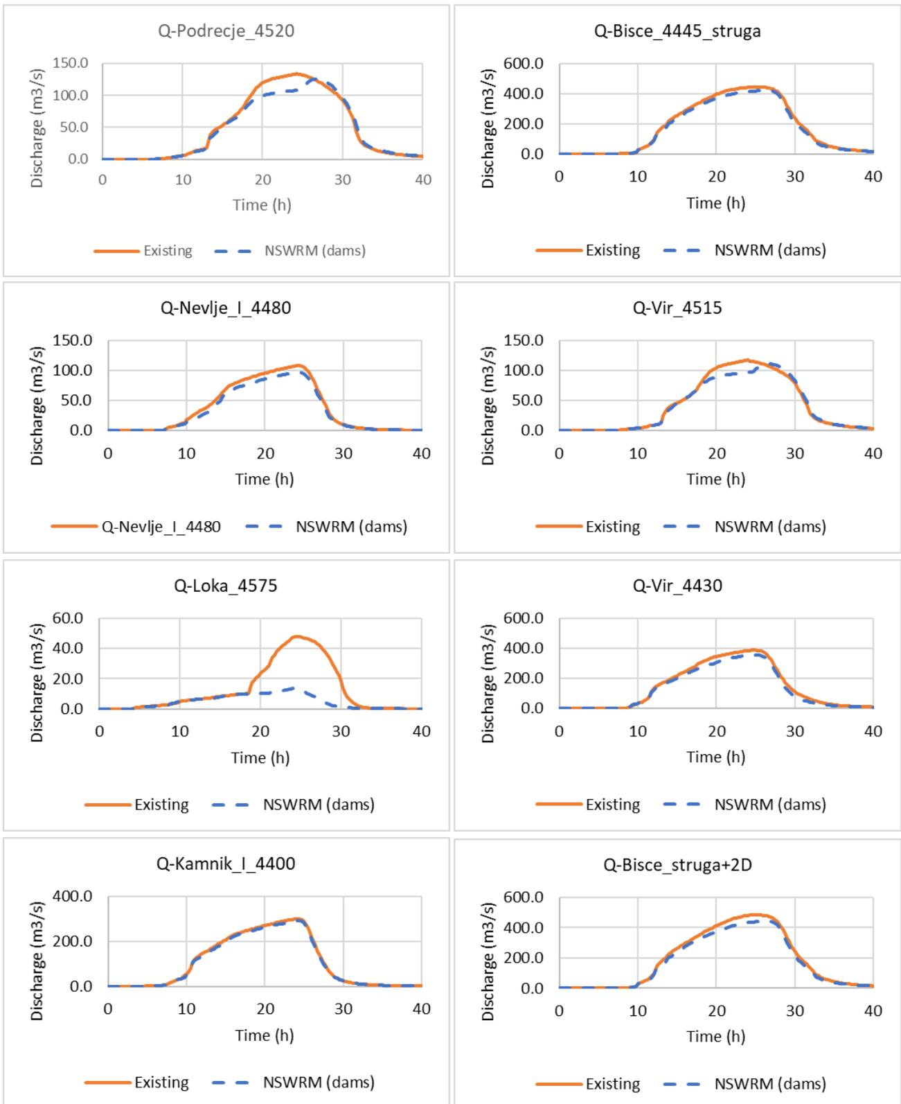
Figure 40: Comparison of computed 24-hour hydrographs with 100-year return period
