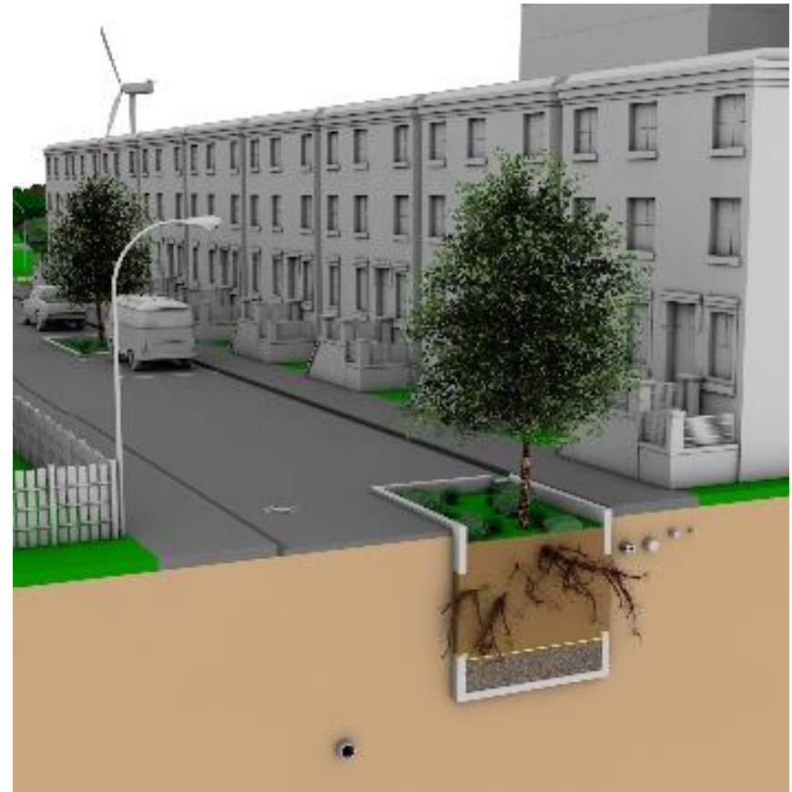
Schematic diagram of a tree-trench system (Source: Sieker)
