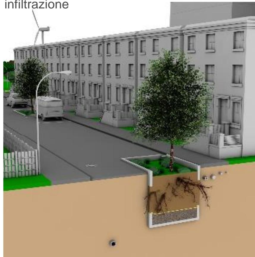
Schematic diagram of a tree-trench system
