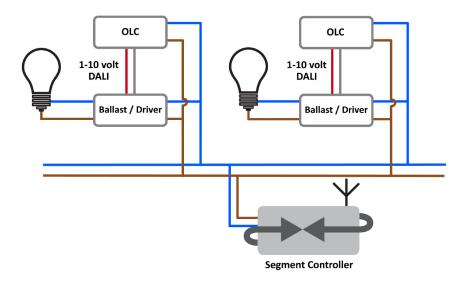
Fig.2.2: Generic architecture of an outdoor adaptive lighting system. From Assessment of framework condition (WP 2 1.9) (p.14) [PDF], by Energy Saving Outdoor Lighting, 2012. Copyright 2010 by Esoli consortium. Retrived from http://www.esoli.org/images/stories/WP\_2\_Final\_Document\_VS\_1.9.pdf. [50]
