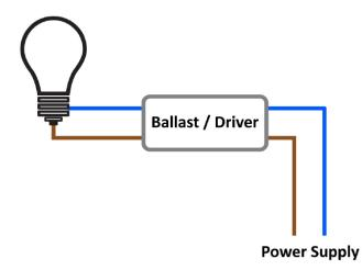
Fig.2.1: Conventional light source and ballast/ driver configuration. From Assessment of framework condition (WP 2 1.9) (p.14) [PDF], by Energy Saving Outdoor Lighting, 2012. Copyright 2010 by Esoli consortium. Retrived from http://www.esoli.org/images/stories/WP\_2\_Final\_Document\_VS\_1.9.pdf. [50]
