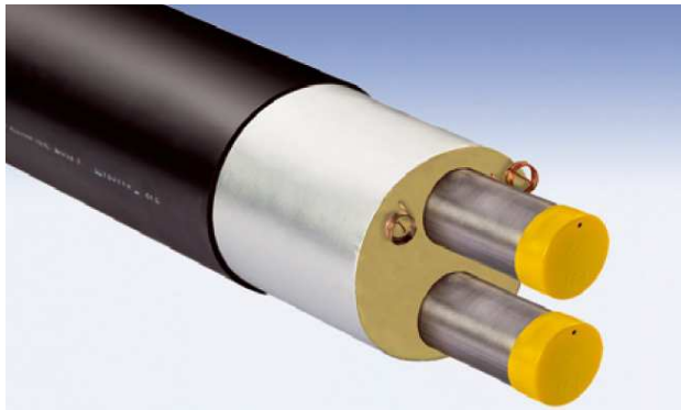
twin steel pipe with PU foam insulation, leak detection, diffusion barrier and plastic jacket
