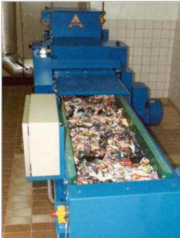
Lab-scale tearing machine
