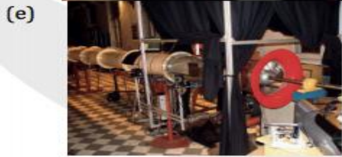
Figure 1(a) CAD model of the axial fan impeller; (b) Axial fan impeller. [2] (c-d) CNC machines at the UB FME: (c) 4-axis; (d) 5-axis. e-f) Test rigs with new experimental equipment at the UB FME: (e) Stereo PIV system; (f) LDA system.
