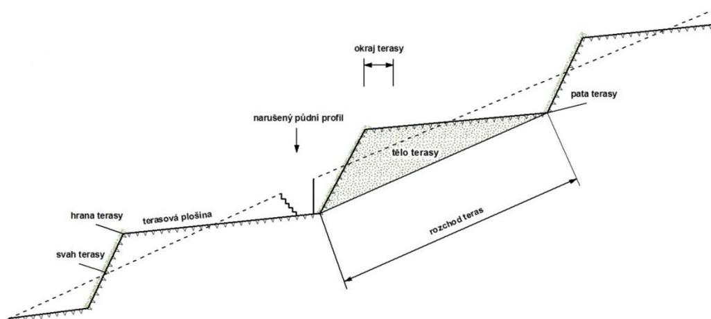
Figure 16: Schematic slope profile with basic description of terraces (source: VÚV TGM, v.v.i.).
