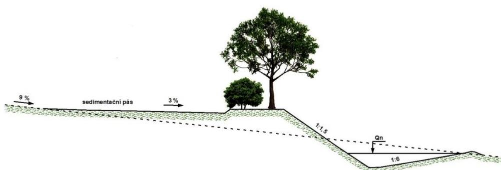
Figure 11: Schemata of basic technical parameters of a baulk in the slope profile (source: VÚV TGM, v.v.i.)
