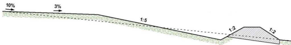
Figure 9: Schemata and basic technical parameters of a dike (source: VÚV TGM, v.v.i.).
