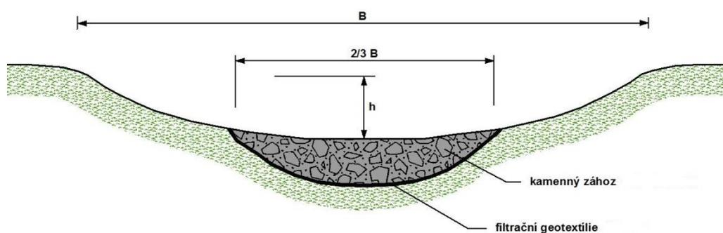
Figure 7: Cross-sectional profile of a stabilization pathway with basic technical parameters (source: VÚV TGM, v.v.i.).
