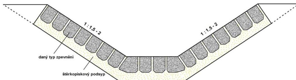
Figure 3: Cross-sectional profile of a ditch with basic technical parameters (source: VÚV TGM, v.v.i.)
