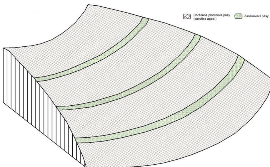
Figure 5: Schematic of an infiltration belt with a longitudinal slope profile (source: VÚV TGM, v.v.i.).
