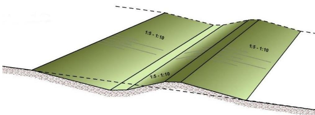
Figure 1: Schematic of the technical design of a furrow. (source: VÚV TGM, v.v.i.)
