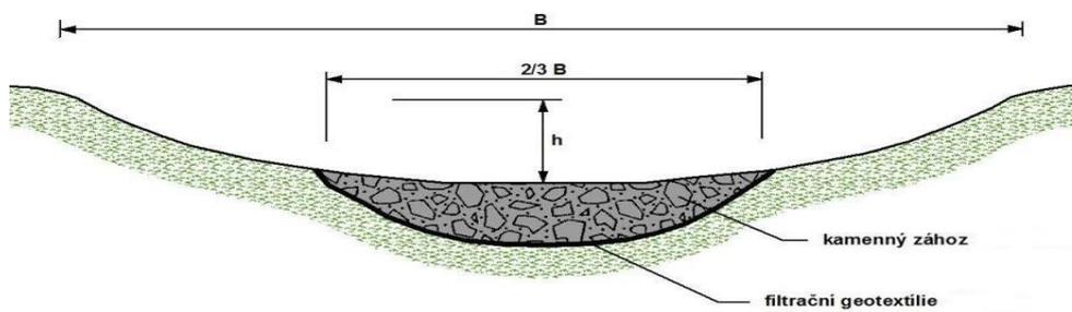
Sample cross section of measure – backfill
