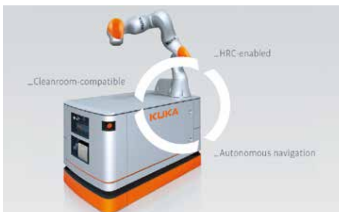
Figure 5 Kuka mobile platform KMR iiwa and robotic arm LBR iiwa
