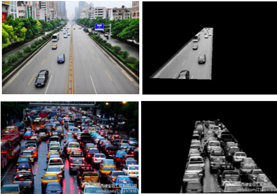
Fig. 15: Statistical analysis of texture in the image with weak (top) and strong (bottom) traffic intensity [8].
