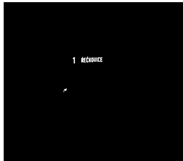
Fig. 17: Example of line number and destination station segmentation using colour space transformation - external vehicle position detection.
