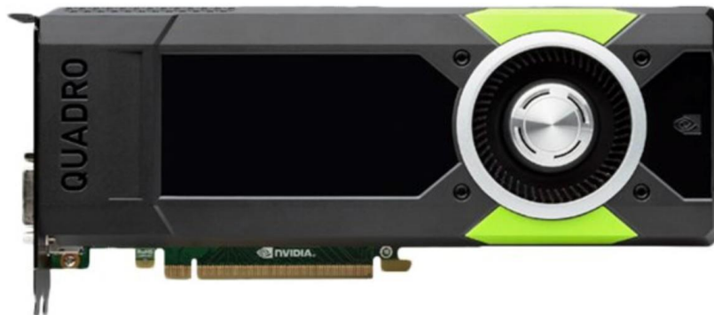
Fig. 41: NVIDIA Quadro M5000 GPGPU with 2048 cores (MC approx. 40 thousand CZK).
