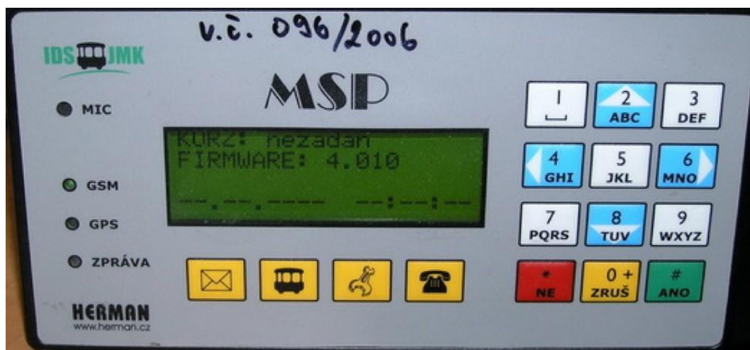
Fig. 11: MSP (Mobile Position Monitoring) terminal of a regional bus [22].
