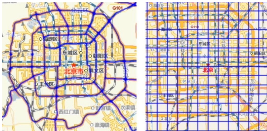
Fig. 25: Traffic map of Beijing city (left) and the division into sectors for congestion indication (right) [9].
