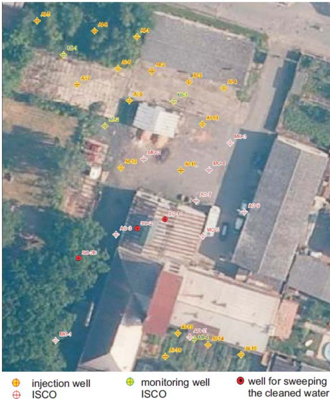
Figure No.9: The network of ISCO wells
