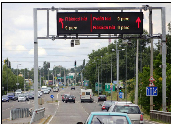
Figure 7 A screenshot of the variable message sign display in Budapest Transport ( www.budapestkozut.hu/forgalomtechnika )
