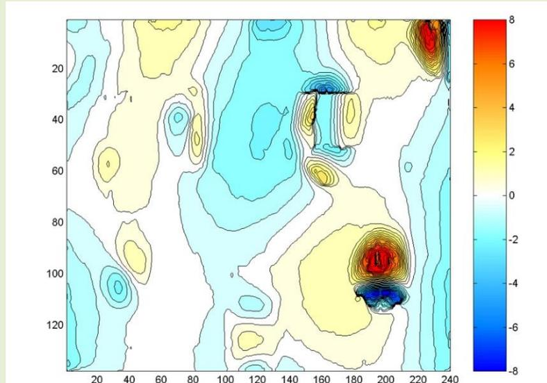
Vibration modes of plaster defects on the test wall at the excitation frequency of 990 Hz (upper) and with a 90° phase shift (lower). The wall was excited mechanically.
