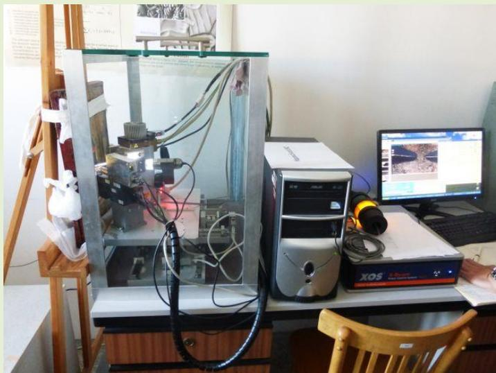
Experimental arrangement of XRF analyzer.
