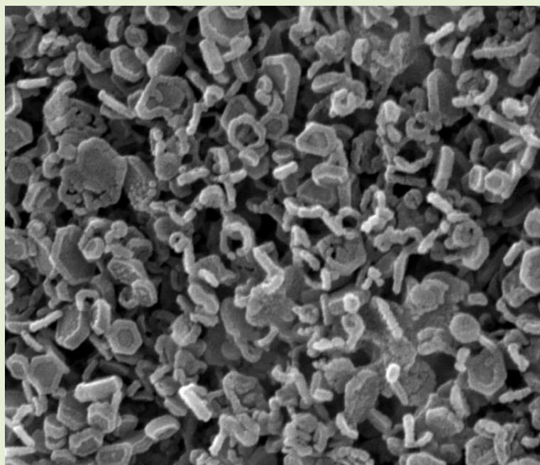
Partially carbonated Ca(OH)<sub>2</sub> nanoparticles observed under SEM.
