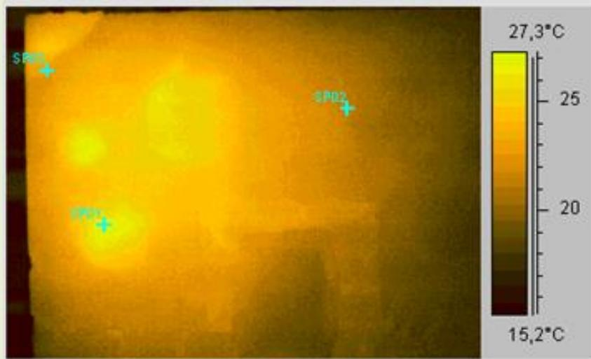
Temperature distribution on the plaster surface (in the central part a mortar plate was fixed along its edges with a deep gap under it). The upper picture shows a situation during external cooling of a pre-heated masonry, the lower the temperatures during external heating of the composed system. Well visible are different material layers, render detachment areas, joints between bricks and fixing mortar under the plate.
