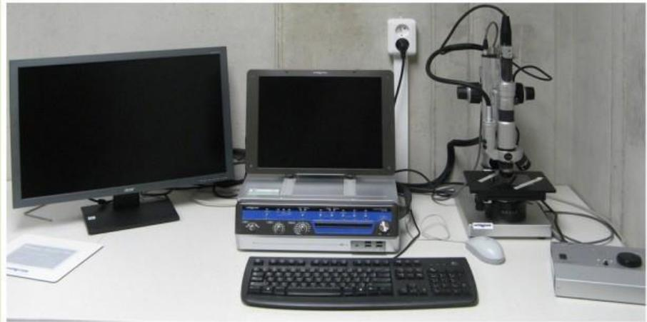
Polarizing microscope, stereoscopic microscope, 3D Digital Video Microscope.
