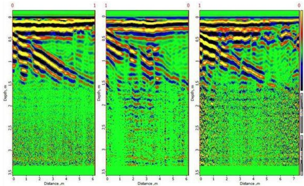
**Tunnel sounding (along). Zond-12e GPR - antenna 500 MHz.**
