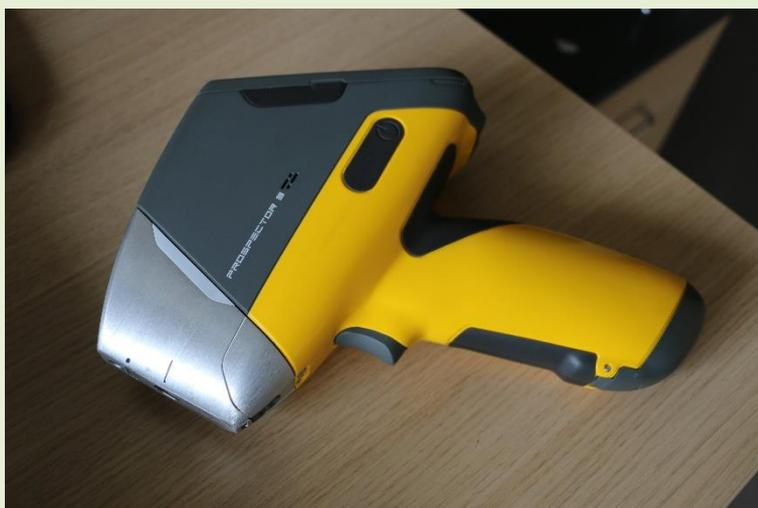
Handheld X-ray fluorescence analyzer.
