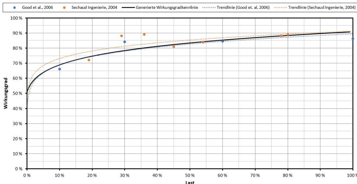
**Figure 18 Generated efficiency curve of the boiler from literature values.<sup>22,23</sup>**
