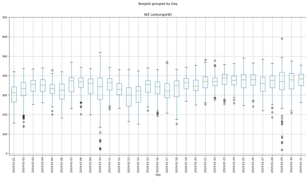
**Figure 9. Snapshot of the load of the local heating network in January 2019.** Circles: outlier, upper whisker:  $1.5 * \text{IQR}$  of box, box top: upper quartile, box middle: median, box bottom: lower quartile, lower whisker:  $1.5 * \text{IQR}$  of box#
