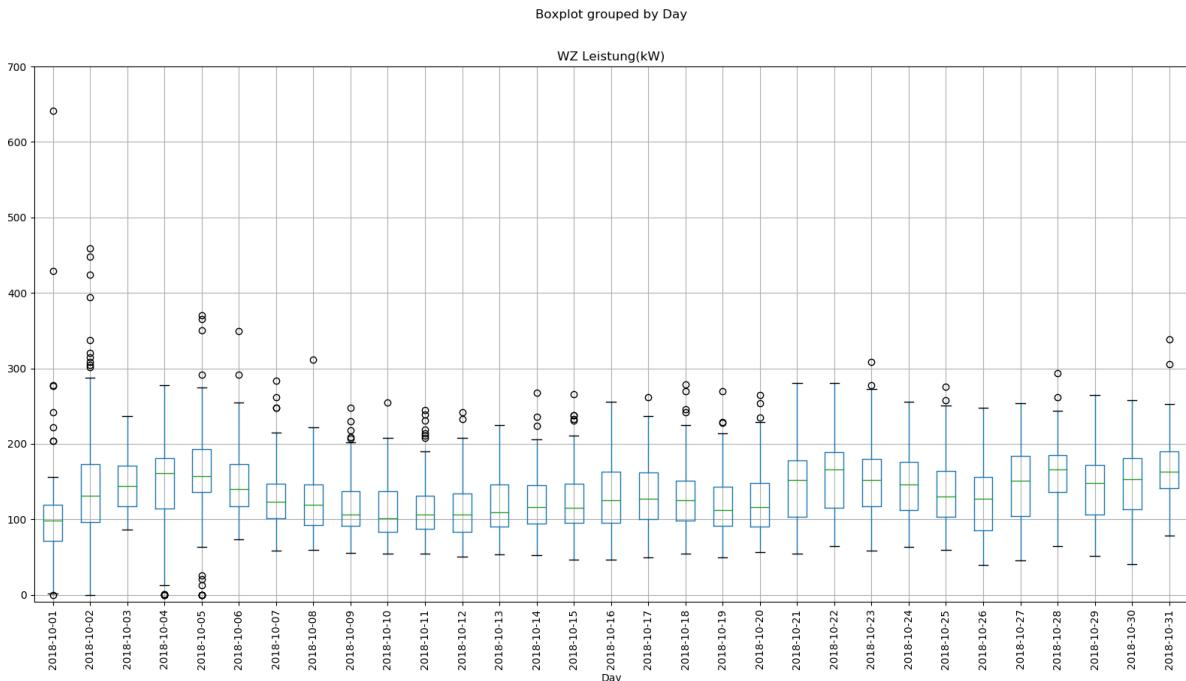
**Figure 7. Snapshot of the load of the local heating network in October 2018.** Circles: outliers, top whisker: 1.5 \* interquartile range (IQR) from box, box top: upper quartile, box middle: median, box bottom: lower quartile, bottom whisker: 1.5 \* IQR from box
