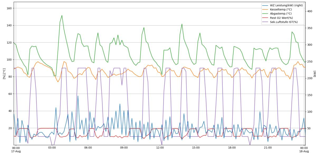
**Figure 5. Various operating parameters of boiler 1 on a typical day in period 1**
