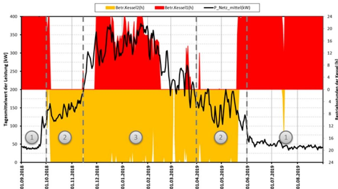
**Figure 4. Daily mean values of the power of the local heating network and operating hours of the two boilers. Red: operating hours, boiler 1. Orange: operating hours boiler 2.**
