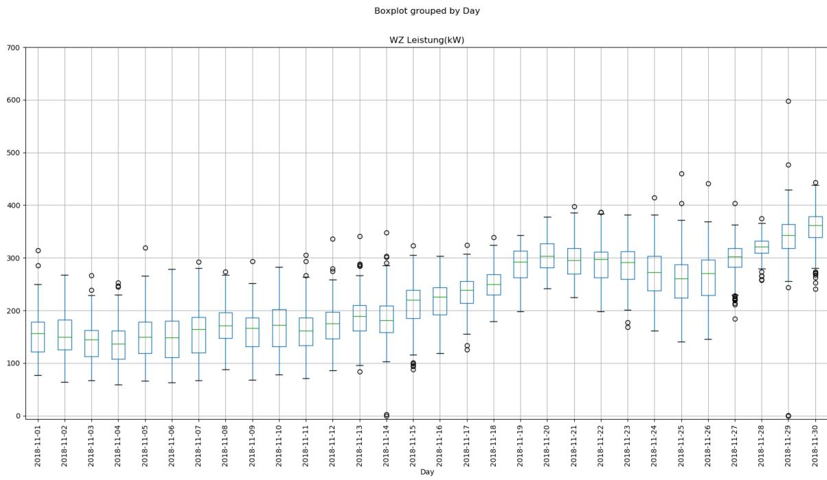
**Figure 8. Snapshot of the the load of the local heating network in November 2018.** Circles: outlier, upper whisker:  $1.5 * \text{IQR}$  of box, box top: upper quartile, box middle: median, box bottom: lower quartile, lower whisker:  $1.5 * \text{IQR}$  of box
