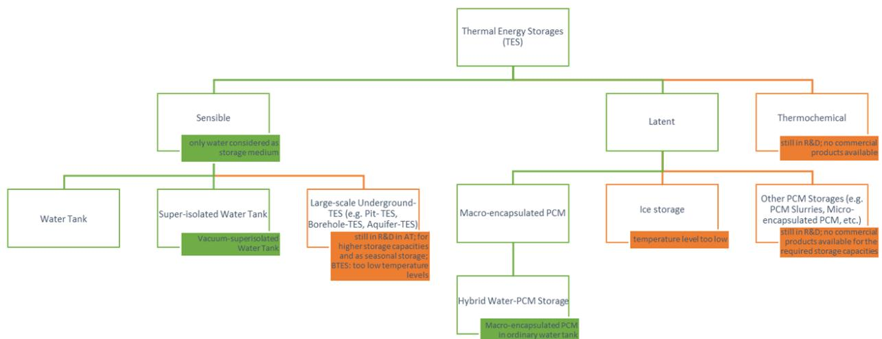
**Figure 13. Storage possibilities for the biomass heating plant Weizberg. Red: Not-feasible. Green: Feasible**
